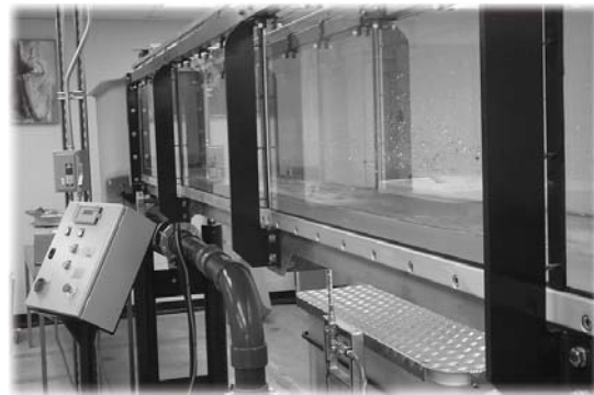
The Armfield S6 MK II flume is a new addition to the department. Students are able to test theories learned in the classroom with this instrument.
