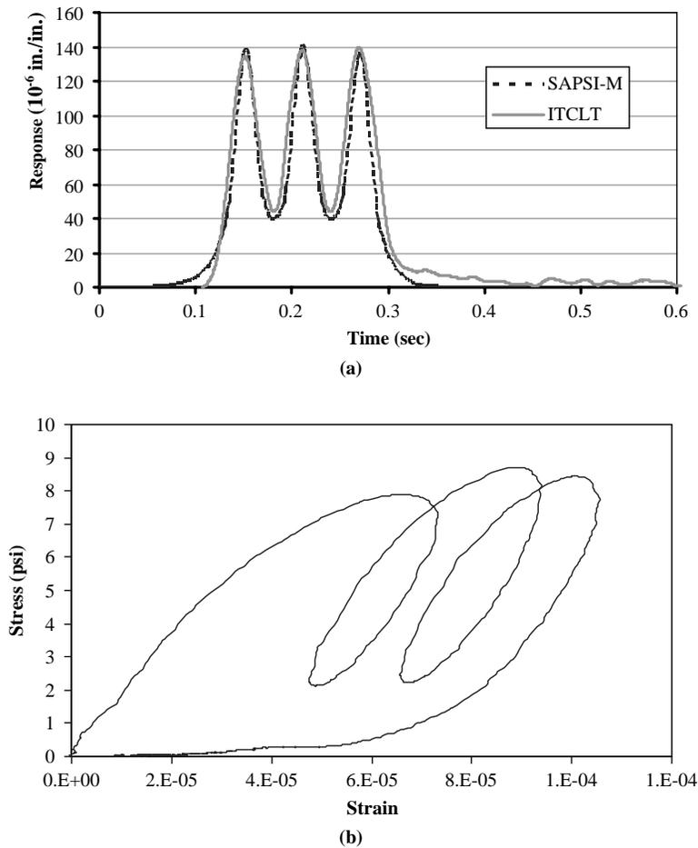
**FIGURE 5** Example strain and stress–strain response curves from cyclic load testing: (a) typical strain pulses from SAPSI-M and indirect tensile cyclic load test (ITCLT) results and (b) typical stress–strain hysteresis loop for tridem axle.
