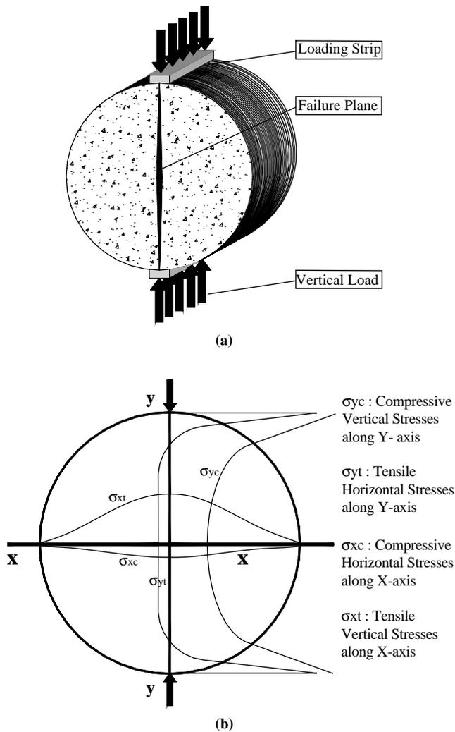
FIGURE 1 Indirect tensile test: (a) indirect tensile loading and (b) stresses in the indirect tensile test specimen.
