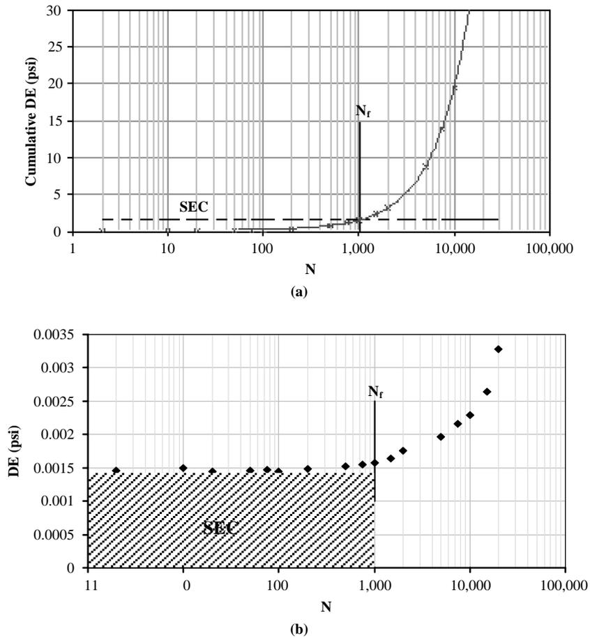
FIGURE 4 Fatigue failure criteria: (a) determining  $N_f$  from cumulative dissipated energy (DE) density and SEC and (b) determining  $N_f$  from dissipated energy density per cycle and SEC.
