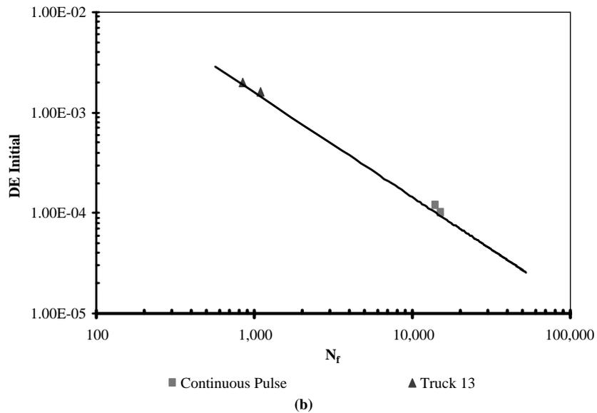
FIGURE 8 Dissipated energy (DE)-based fatigue curve: (a) fatigue curve using various axle configurations and (b) fatigue responses under pulse load and truck.
