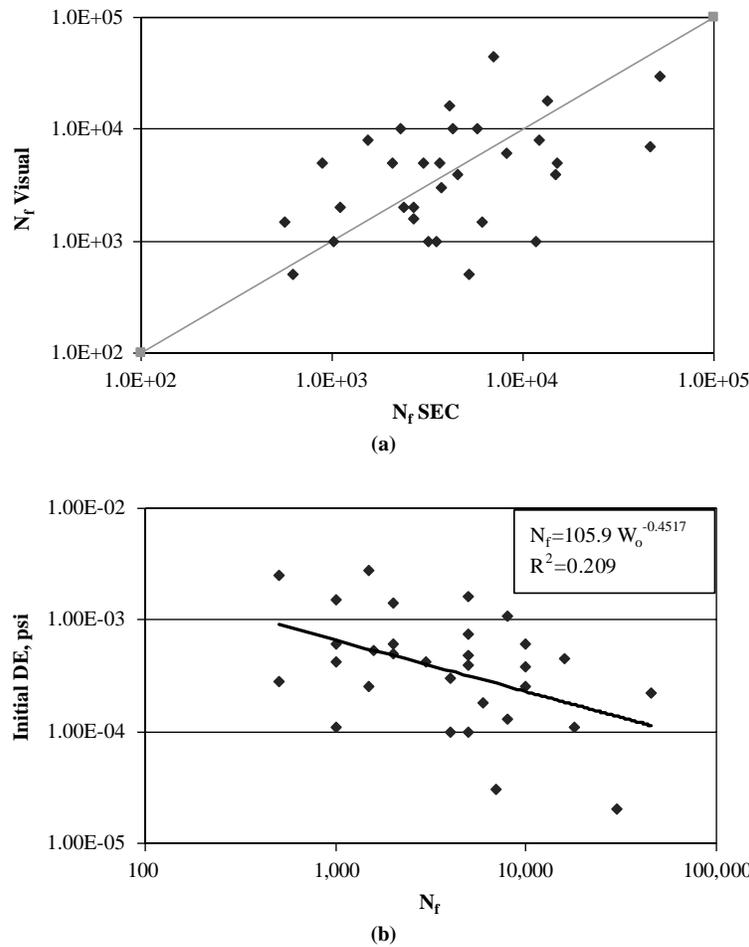
FIGURE 7 Comparisons of visual and SEC failure criteria: (a)  $N_f$  based on visual criteria and SEC and (b) fatigue curve based on visual criteria (DE = dissipated energy).
