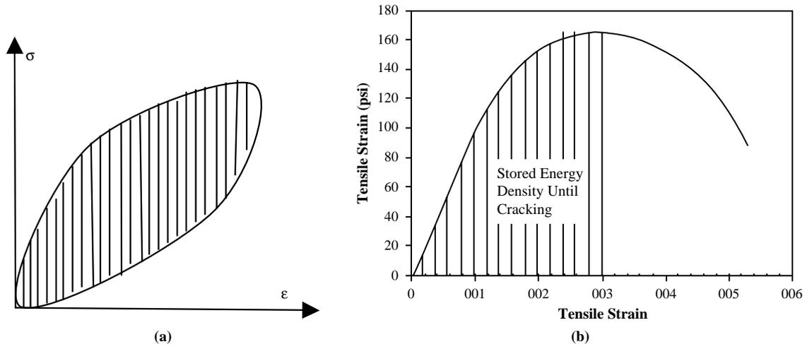
FIGURE 3 Stress-strain relationships under cyclic load and strength testing: (a) dissipated energy density under cyclic load testing and (b) stored energy density until failure under strength testing.
