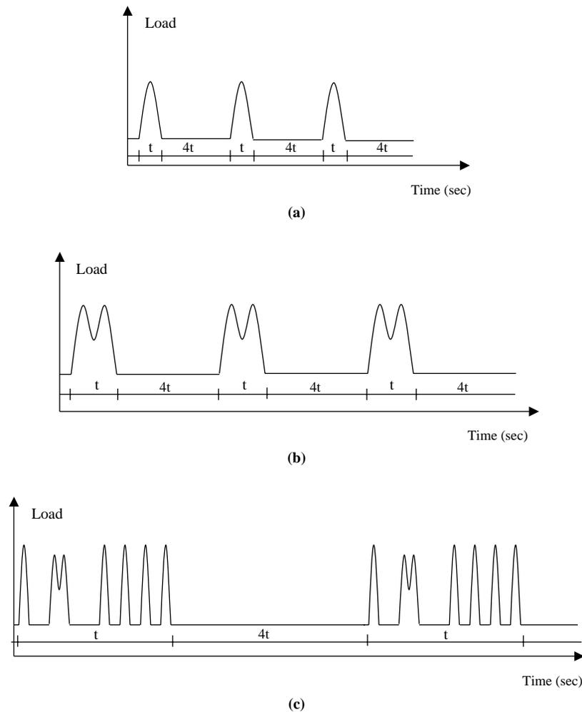
FIGURE 6 Examples of load cycles used in fatigue testing: (a) single axle, (b) tandem axle, and (c) Truck 10 ( $t$  is the duration of loading pulse and  $4t$  is the rest period).
