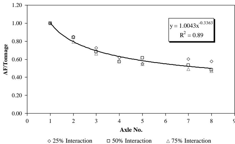
FIGURE 9 Axle factors per tonnage for different interaction levels.
