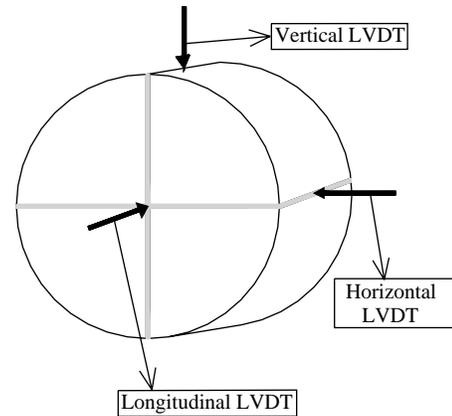
FIGURE 2 LVDT configurations for indirect tensile cyclic load.
