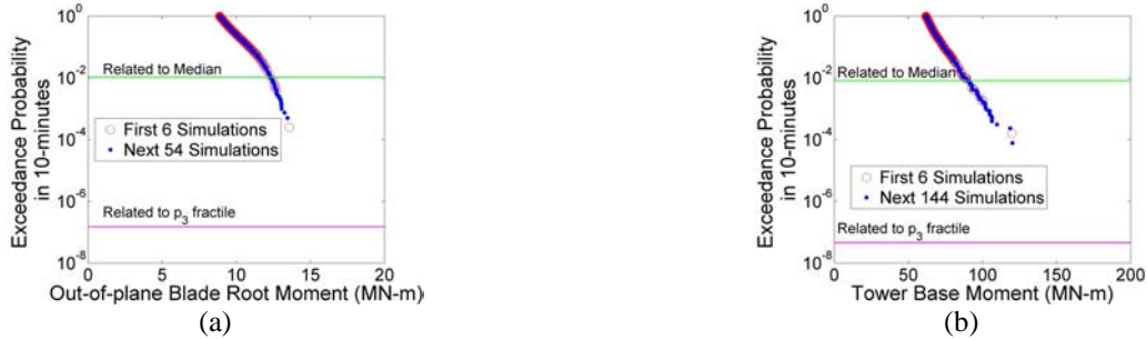
Figure 8. Load distributions of the POT data for governing environmental states based on (a) 60 simulations of OoPBM for a mean wind speed of 14 m/s and a significant wave height of 5.5 m; and (b) 150 simulations of TBM for a mean wind speed of 16 m/s and a significant wave height of 5.5 m.
