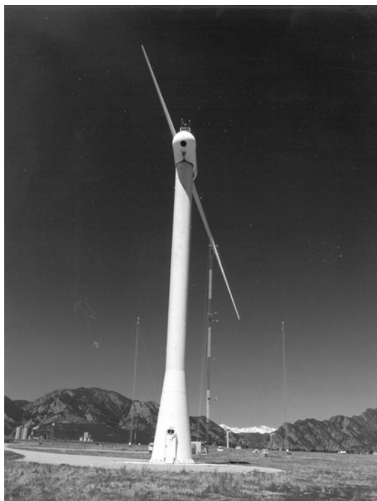
Figure 1. The Turbine and the 42-m Inflow Measurement Array Upwind of the Turbine.
