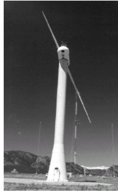
Figure 1. The National Wind Technology Center’s Advanced Research Turbine (ART) used in the numerical studies.
