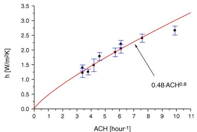
Fig. 8. Experimental data with uncertainties compared to the new equation for the convection correlation for floor surfaces with DV diffuser (exponent,  $m = 0.8$ ).
