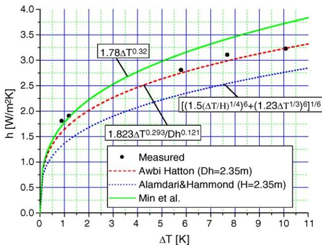
Fig. 11. Validation of the existing natural convection correlations with the measured data for vertical wall surfaces in a room with DV.
