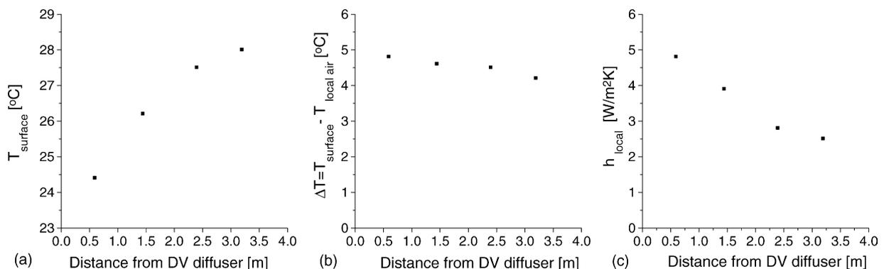
Fig. 6. Variation of temperatures and local convection coefficients with horizontal distance from the DV diffuser. The measurements were at the diffuser centerline and 0.1 m above the floor. The supply temperature was 17.9 °C and volume airflow rate provided 4.6 ACH in the climate chamber: (a) surface temperature distribution; (b) local temperature differences; (c) local convection coefficients.
