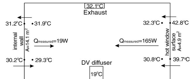
Fig. 12. Measured temperature and heat fluxes in the experimental facility with the hot window surface and the internal wall on the opposite side.
