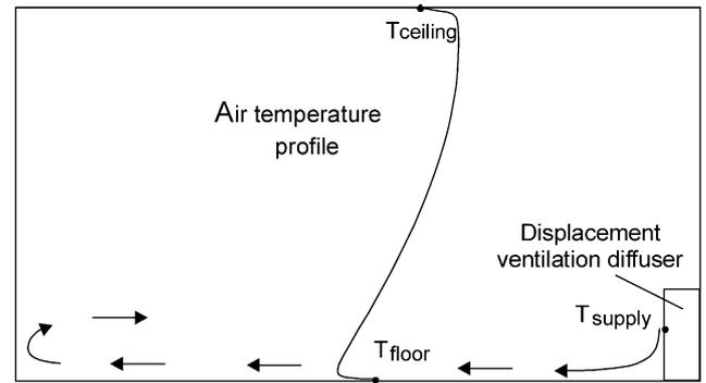
Fig. 1. A characteristic airflow pattern and temperature stratification in a room with displacement ventilation.
