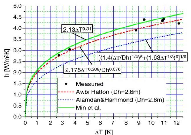
Fig. 10. Performance of the existing natural convection correlations and measured data for floor surfaces, where  $T_{floor} > T_{air}$ .
