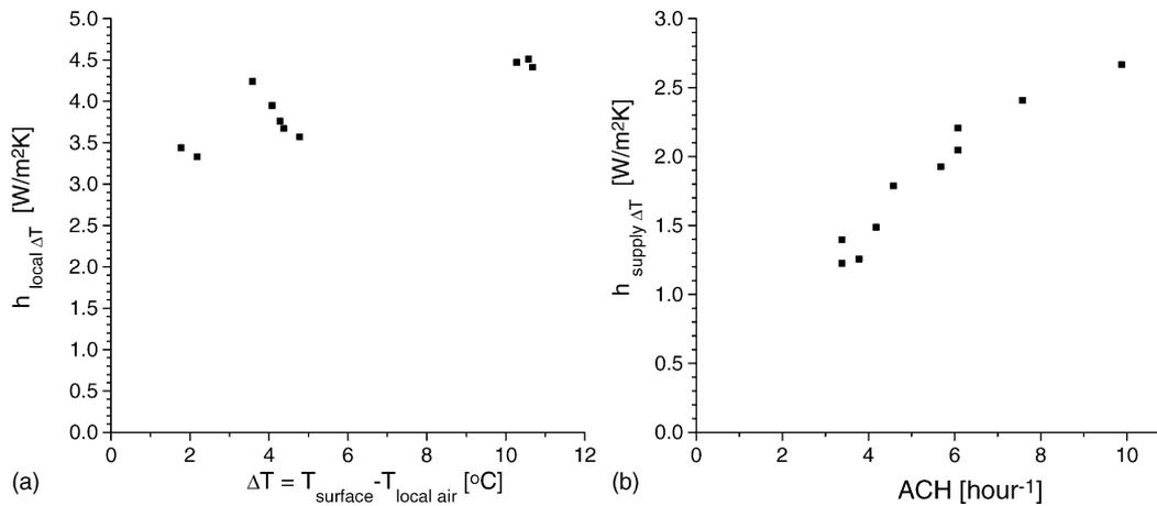
Fig. 7. Measured convection coefficients ( $h$ ) for the floor with displacement ventilation as a function of a local temperature difference ( $\Delta T$ ) and the supply flow rate (ACH): (a)  $h$  as a function of  $\Delta T$  and (b)  $h$  as a function of ACH.
