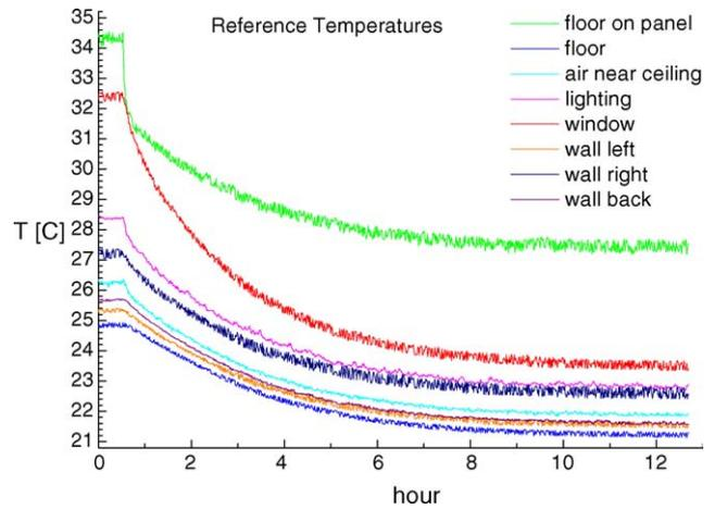
Fig. 5. An example of temperature recording for determination of steady-state conditions in the environmental chamber for natural convection validation.
