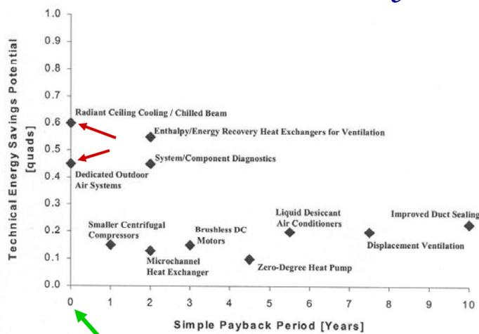
Figure 5-2: Estimated Technical Energy Savings Potential and Simple Payback Periods for the 15 Options
