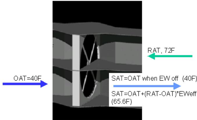
By adjusting the EW ON time (54.7% or 8.2 min) in 1 period (15 min) can get an avg. temperature equal to the desired SAT (54F). Duty cycle changes to 100% ON at 40F OAT to avoid tripping freeze stats.
