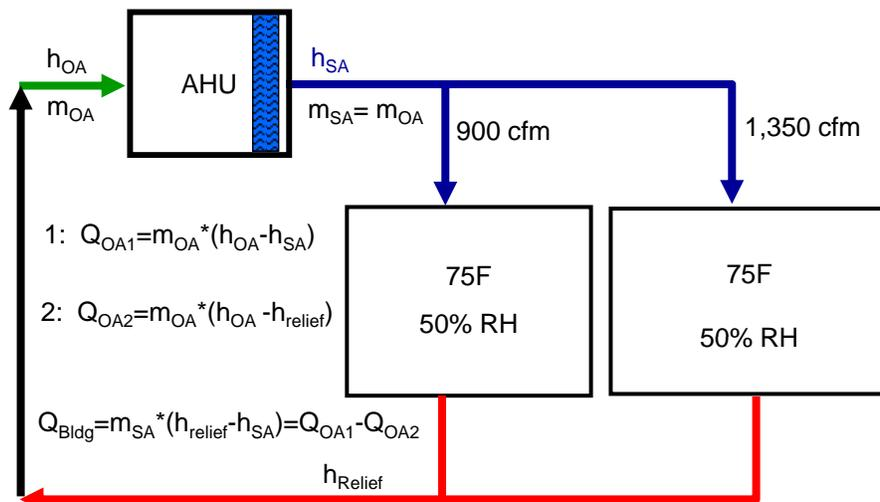
So,  $Q_{OA2}$  is correct:  $Q_{OA1} = Q_{OAcorrect} + Q_{Bldg} = \text{coil load}_{72}$
