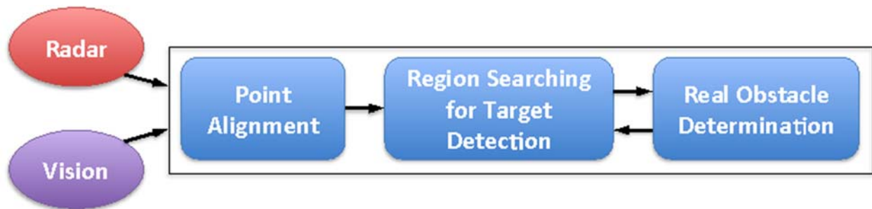
Figure 3.3: Fusion with mmWave radar [38]
