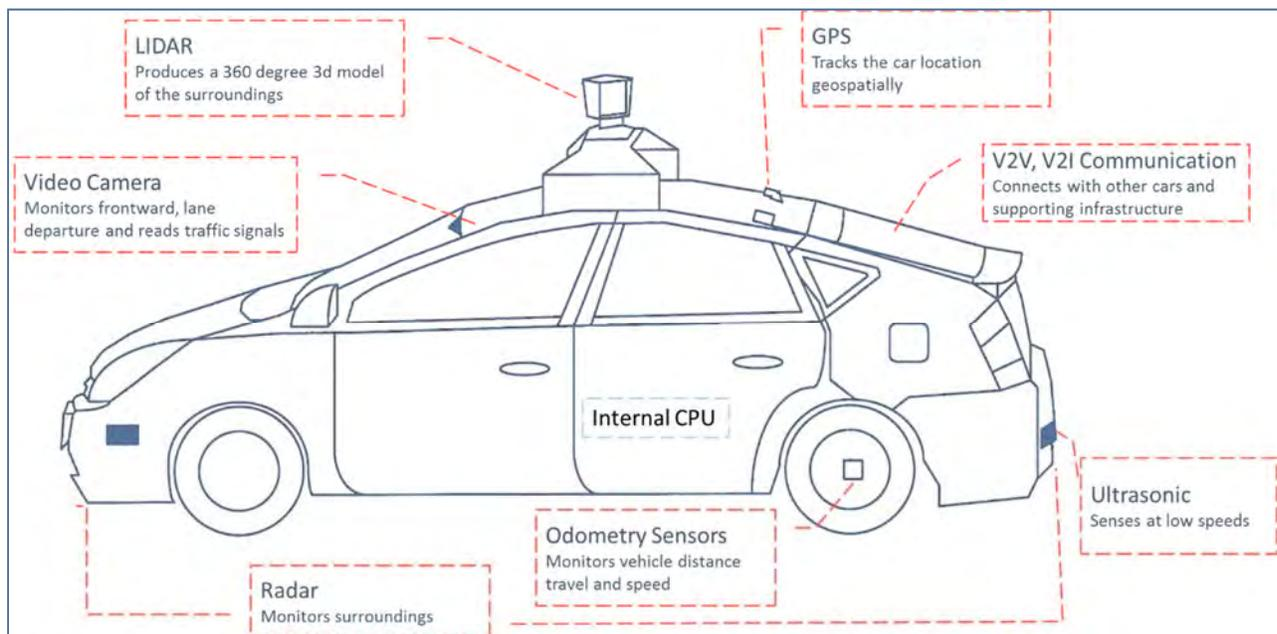
Figure 2: Autonomous Vehicle Sensor Suite (3).
