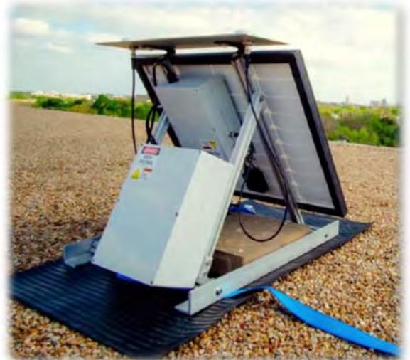
*Figure 10: A stationary differential GPS unit deployed by researchers at the University of Texas (18).*
