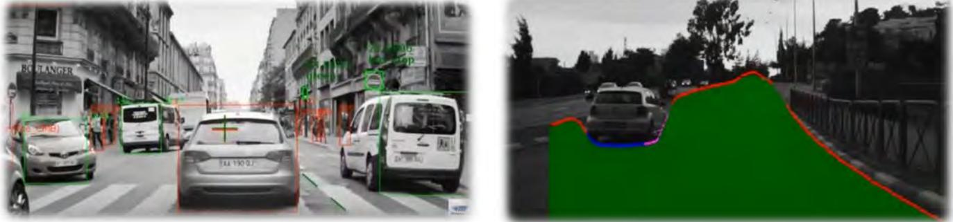
Figure 11: Camera-based object and sign detection and clear space detection (20).
