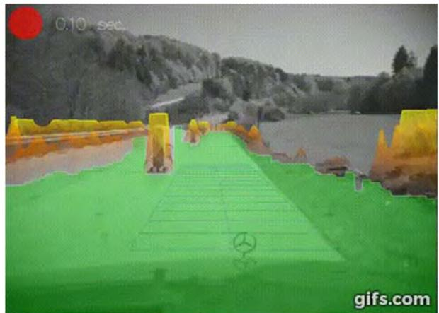
Figure 16: Grid-based Occupancy Mapping (34).
