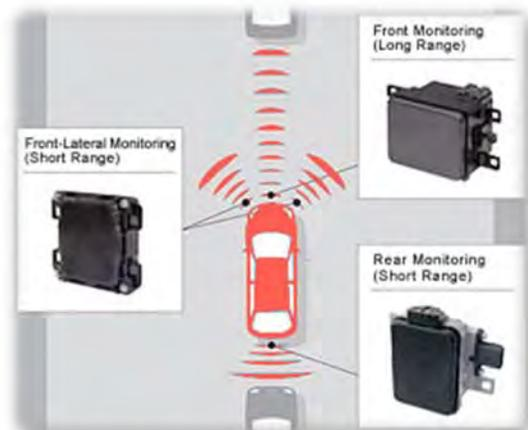
Figure 12: Radar systems in AVs (24).
