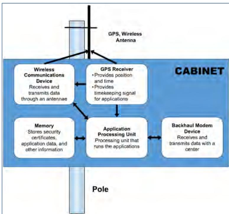
Figure 28: Overview of RSU Functions (51).
