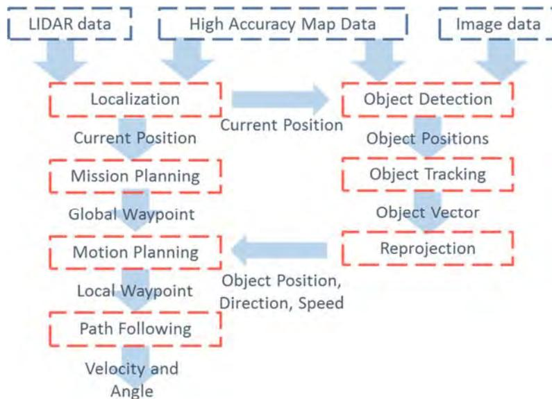
Figure 14: LIDAR Dependent Software Process(31)
