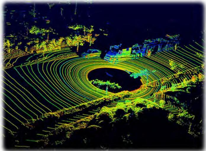
Figure 6: 64-laser LIDAR point cloud (5).
