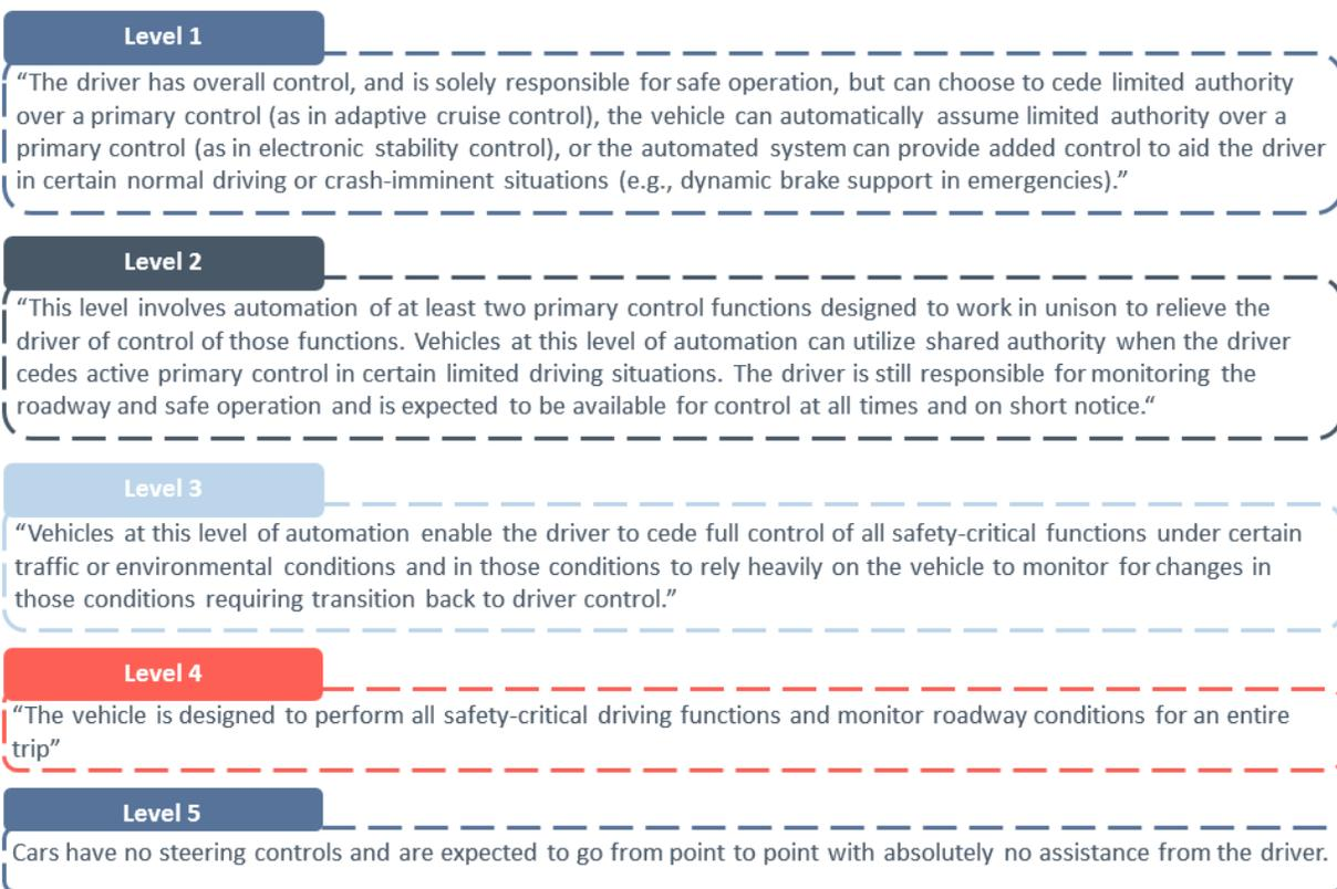
Figure 1: SAE Levels of Automation (2).
