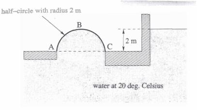
For the shown half-cylindrical gate, ABC, of radius of 2 meters and width of 5 meters determine (consider water at 20° Celsius):
