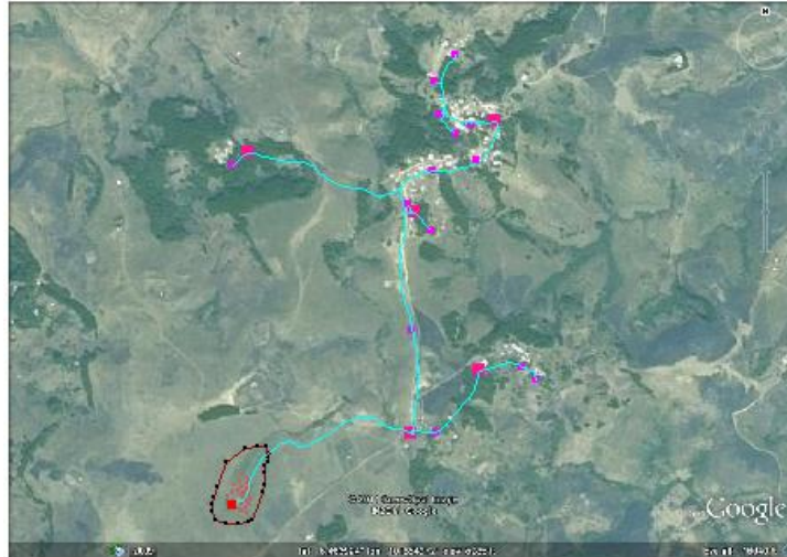
Figure 1. GoogleEarth image of Ntisar Village, Cameroon. The blue line represents the pipeline, the large pink boxes are the storage tanks, the small pink boxes the public tap stands, the red large box is the spring box, the small red boxes (in the polygon) are the monitoring wells, and the brown polygon represents the fence that was built surrounding the catchment. The length of the box shown is ~3 km.
