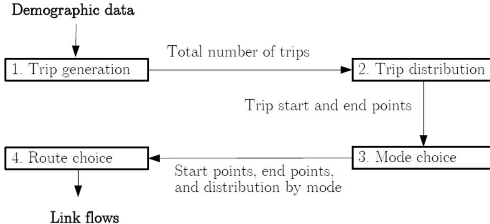
Figure 2: Schematic of the four-step process.
