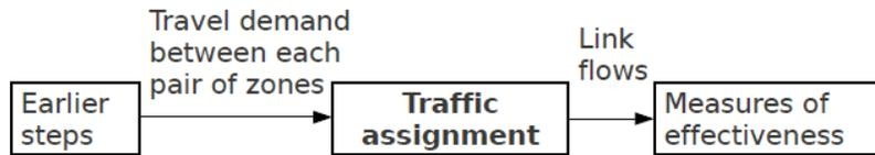
Figure 3: Inputs and outputs of traffic assignment.
