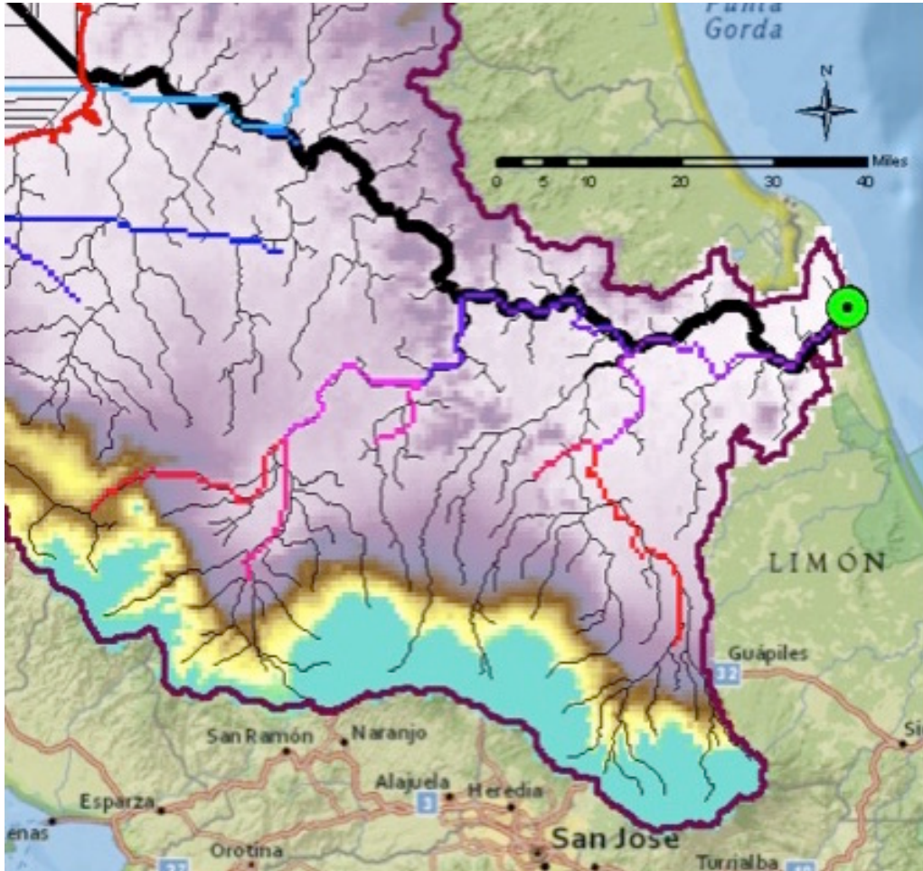
Figure 8 The delineated streams do not accurately represent the river network that drains Lake Nicaragua.
