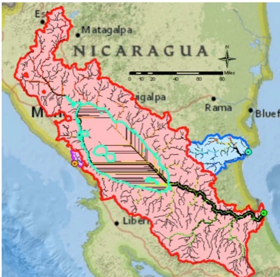
Figure 24 Complete delineated basins that the canal could potentially affect
