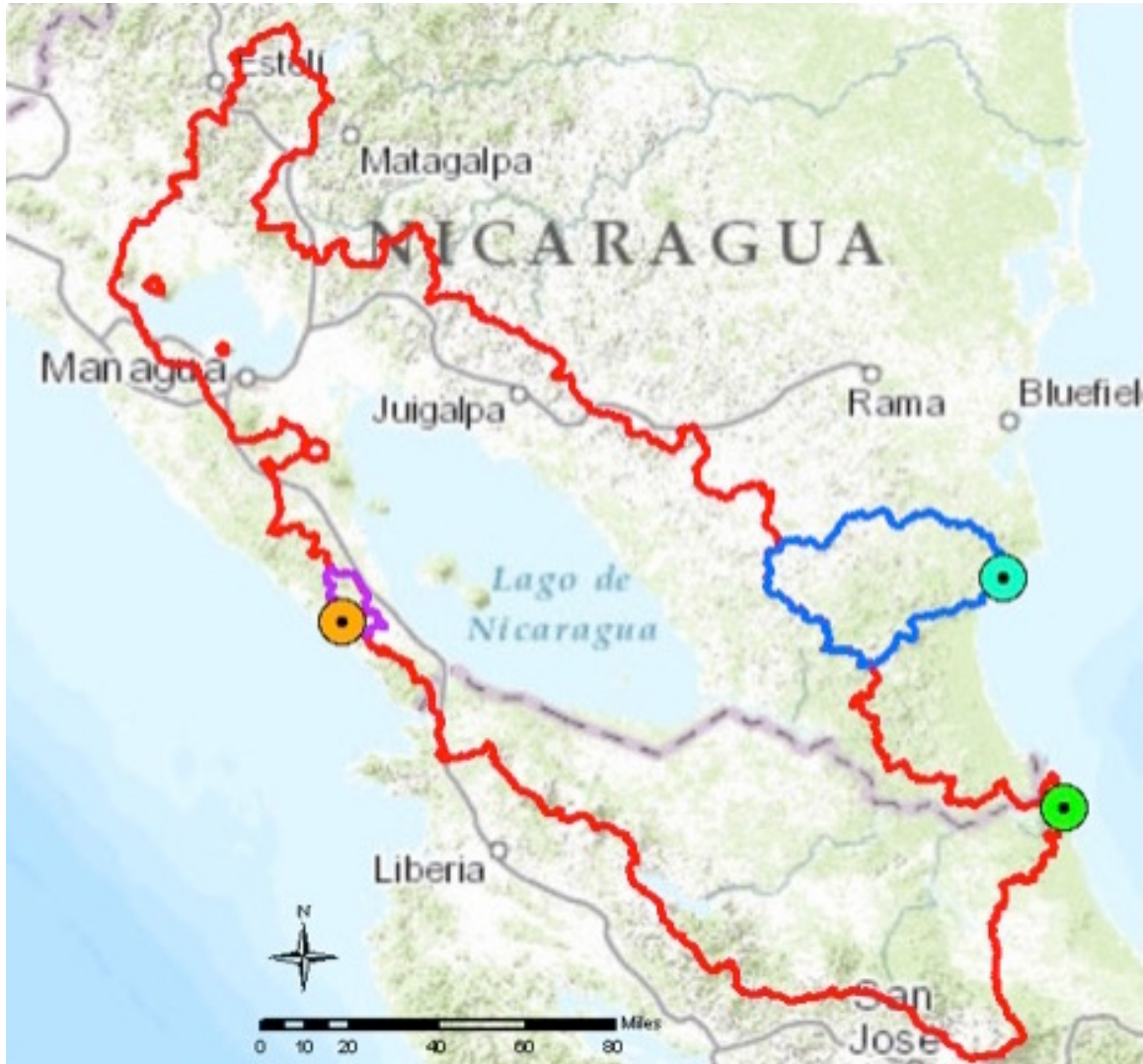
Figure 2 The proposed canal will stretch from Brito to Punta Gorda, stretching across three drainage basins.
