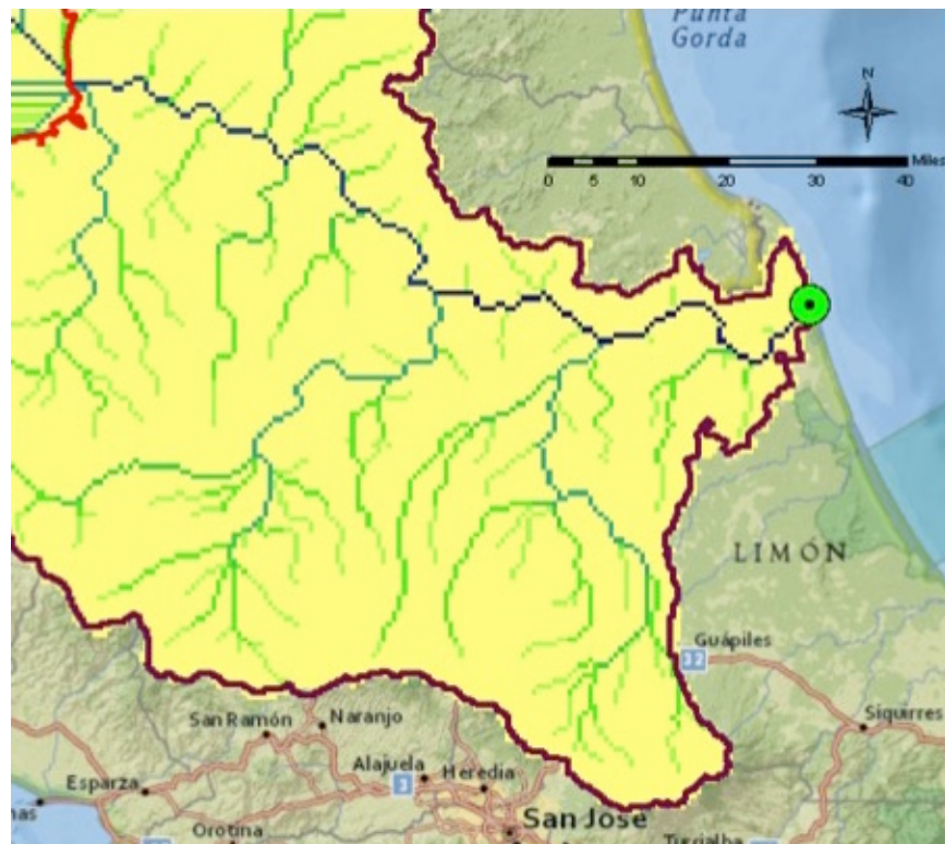
Figure 21 The flow accumulation from the reconditioned DEM shows the connected streamlines
