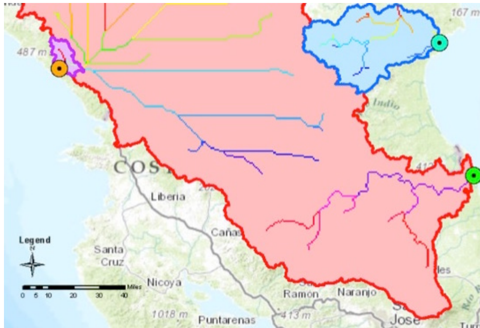
Figure 7 Delineated streamlines in the basins illustrated using the Raster Calculator and Stream Link tools.
