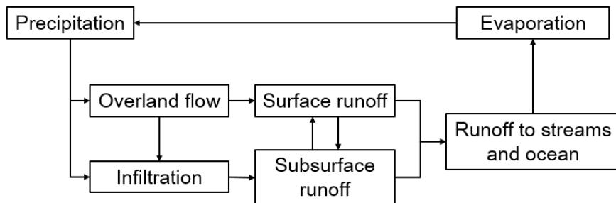
Figure 3 Simplified hydrologic cycle adapted from Chow et al. (1988)
