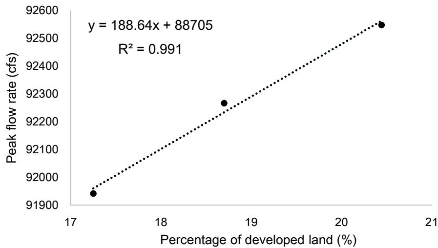
Figure 18 Linear fitting of the relationship between percentage of developed land and peak flow rate
