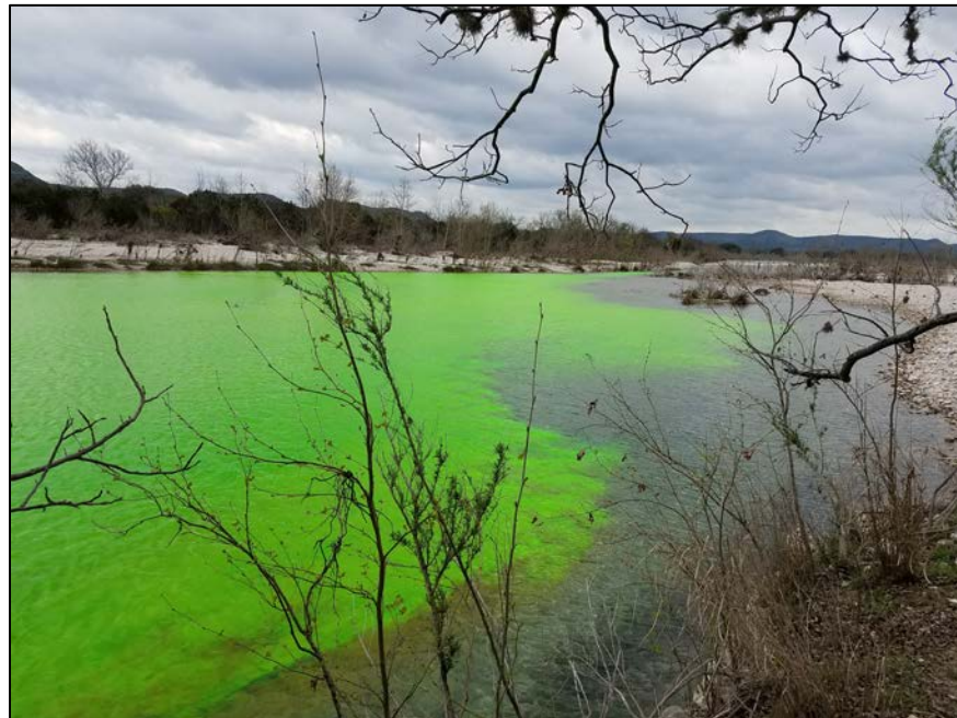
Figure 16. Uranine dye immediately downstream of the injection point on the Nueces River, March 2017. The non-toxic, fluorescent dye is used to investigate subsurface velocities.
