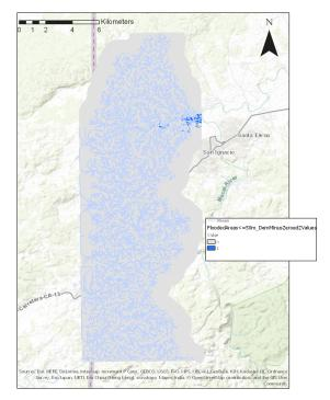
Figure 15: Incorrect flood inundation map for flood stage of 50m using beta method of HAND mapping, stream elevations set to 0
