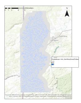
Figure 14: Incorrect flood inundation map for flood stage of 6m using beta method of HAND mapping, stream elevations set to 0
