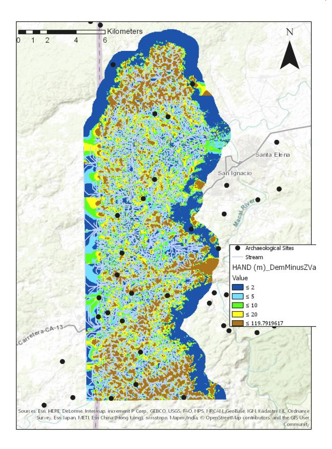
Figure 6: Beta method of HAND mapping, including only values greater than 0
