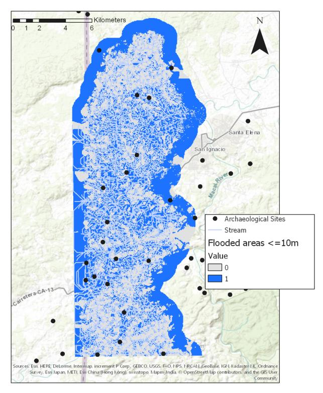
Figure 19: Flood inundation map for flood stage of 10m using beta method of HAND mapping, including only values greater than 0
