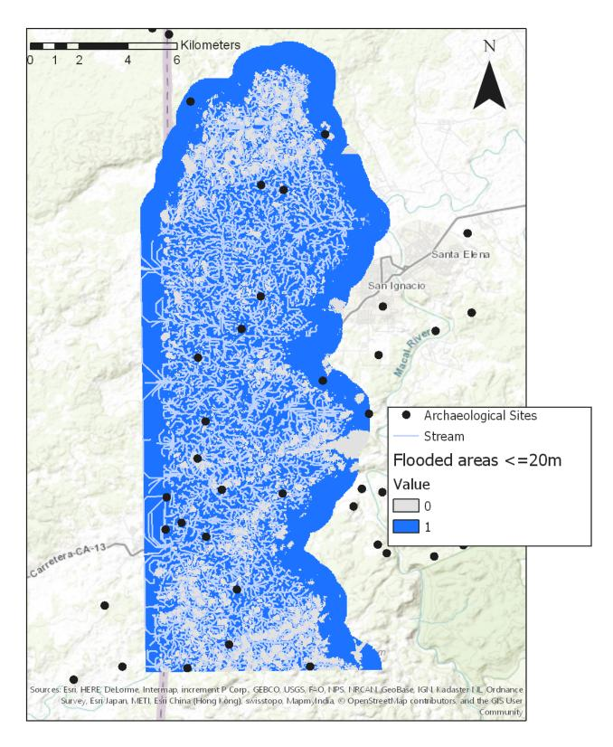
Figure 21: Flood inundation map for flood stage of 20m using beta method of HAND mapping, including only values greater than 0
