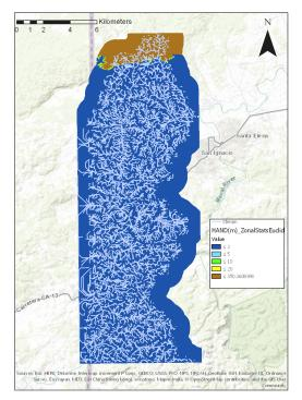
Figure 13: Incorrect HAND map produced from Zonal Statistics and Euclidean Allocation
