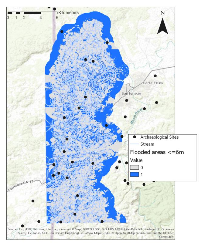
Figure 18: Flood inundation map for flood stage of 6m using beta method of HAND mapping, including only values greater than 0
