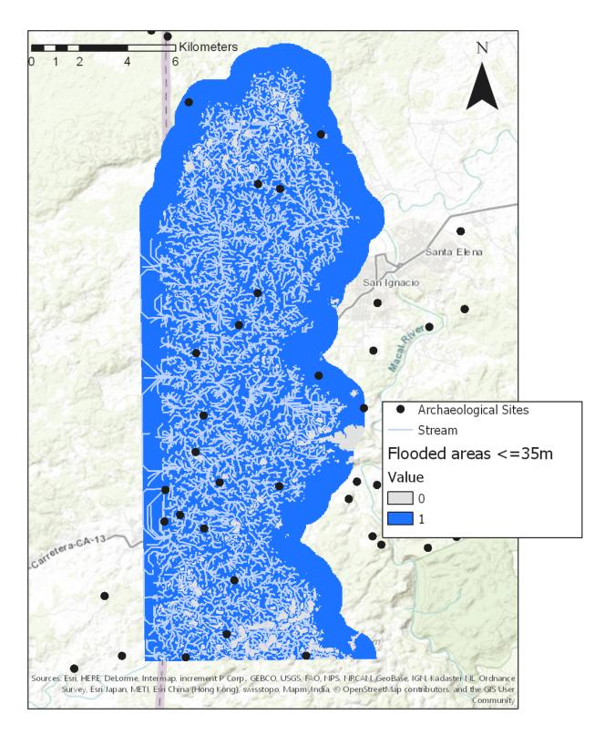
Figure 22: Flood inundation map for flood stage of 35m using beta method of HAND mapping, including only values greater than 0
