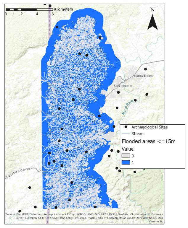
Figure 20: Flood inundation map for flood stage of 15m using beta method of HAND mapping, including only values greater than 0
