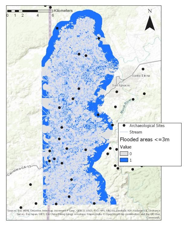
Figure 17: Flood inundation map for flood stage of 3m using beta method of HAND mapping, including only values greater than zero
