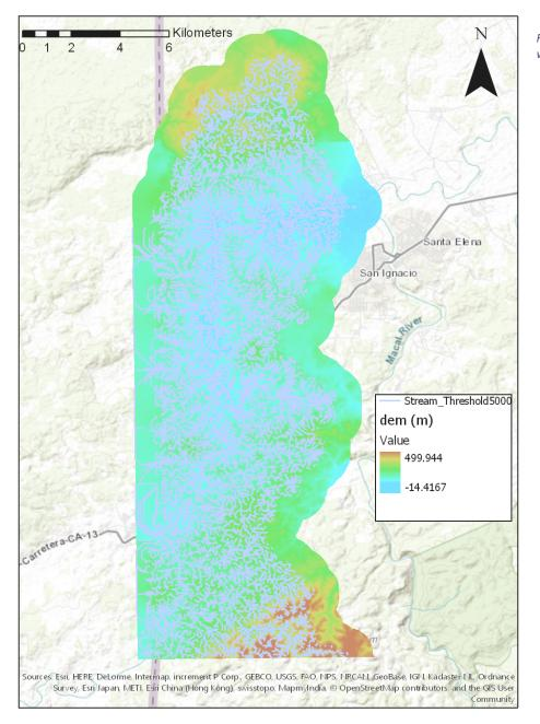
*Figure 3: Stream network with threshold of 5,000*
