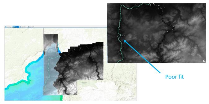
Figure 11: Poor agreement between streams delineated from SRTM imagery and my LiDAR DEM
