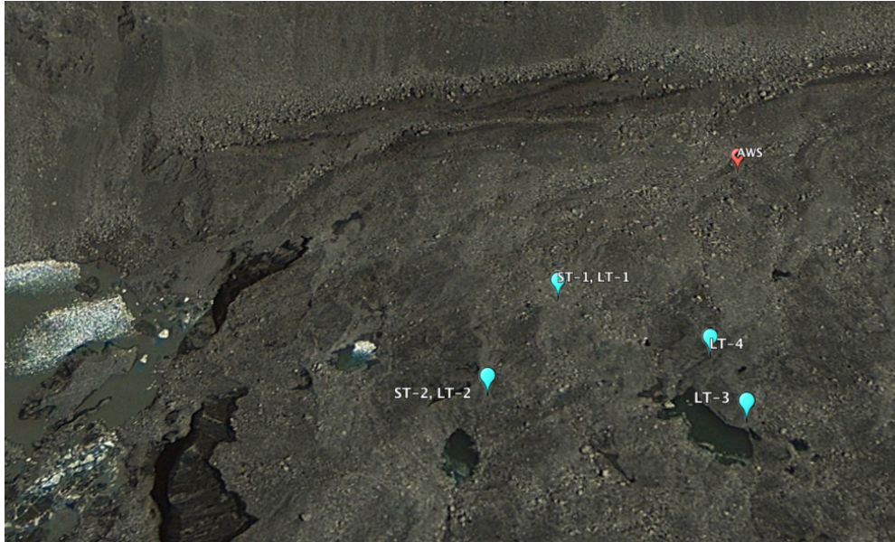
Figure – Location of temperature sensors and weather station at Imja glacier.
