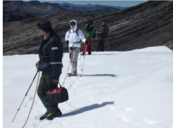
Figure 4. Conducting GPR survey on Pastoruri glacier.
