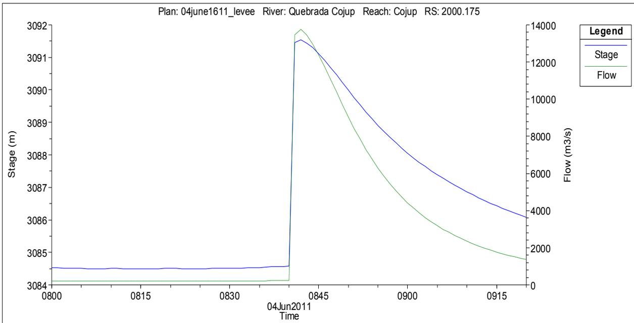
**Figure 6: Downstream cross section hydrograph**
