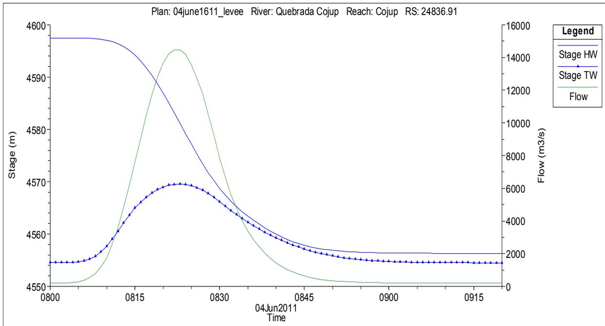
**Figure 5: Dam breach hydrograph. HW: headwater, TW: tailwater**
