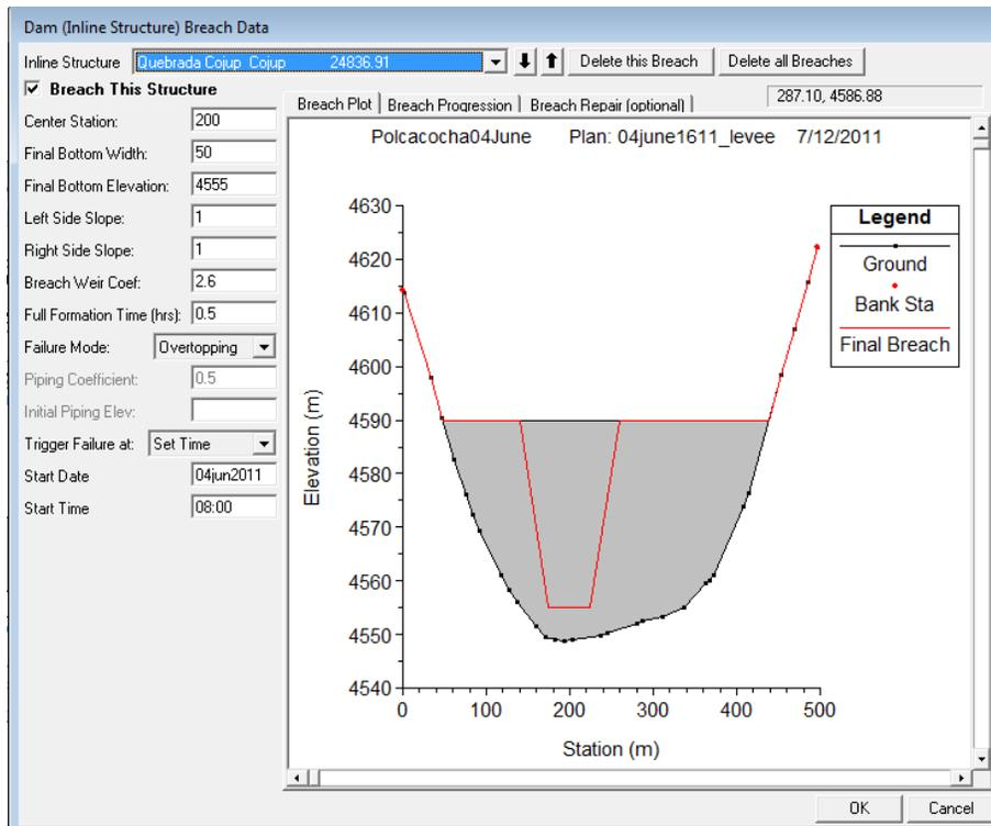
**Figure 11: Dam breach input data.**
