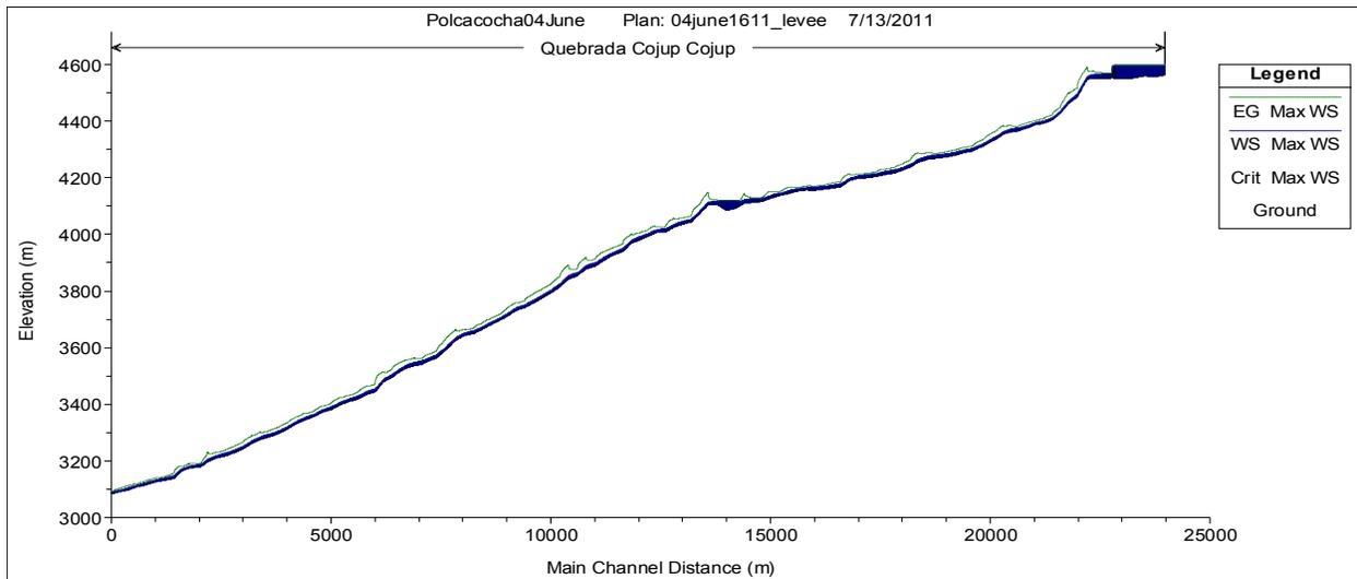
**Figure 7: Longitudinal profile of the maximum flow.**
