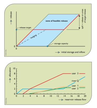
**Figure 3.3.** Policy defining the reservoir release to be made as a function of the current storage volume and current inflow and the reservoir release allocation policy for the river flow downstream of the reservoir. The blue zone in the reservoir release policy indicates the zone of feasible releases. It is physically impossible to make releases represented by points outside that blue zone.
