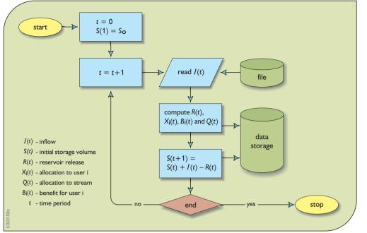
Figure 3.4. Flow diagram of the reservoir-allocation system simulation process. The simulation terminates after some predefined number of simulation time steps.
