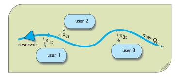
Figure 3.2. Reservoir-water allocation system to be simulated.
