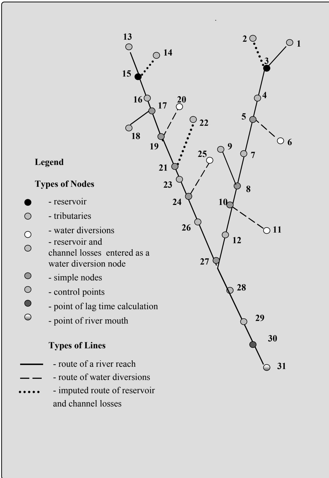
**Figure 1. The Schematic of a Test Reach of the Syr Darya River.**
