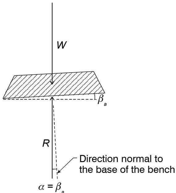
**Figure 4. Forces acting on an anchor bench when there is no wind.**
