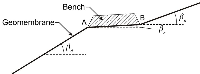
**Figure 3. Anchor bench geometry.**
