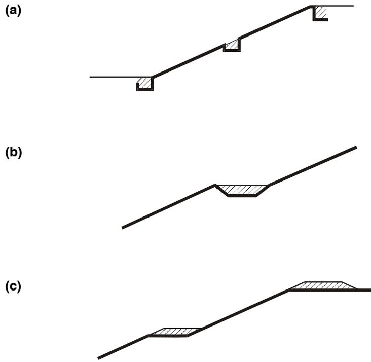
Figure 2. Examples of anchor trenches (a, b) and benches (c).
