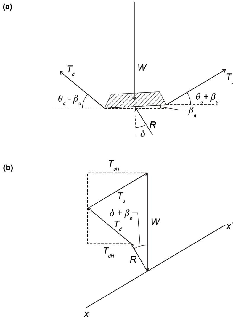
Figure 8. Case of anchor bench failure by sliding in the upslope direction: (a) forces acting on the anchor bench; (b) force diagram.
