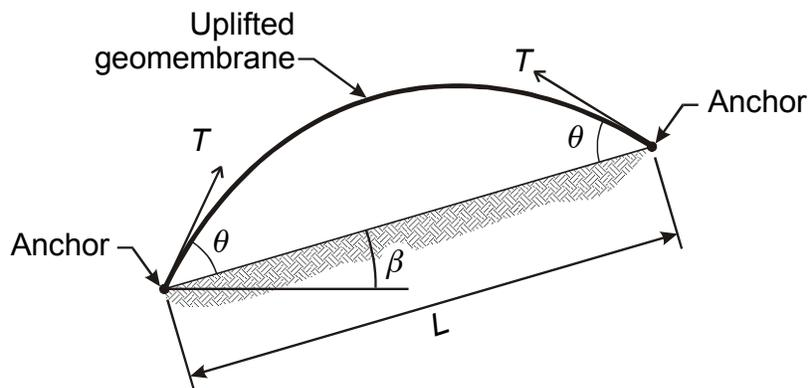
Figure 1. Configuration of an uplifted geomembrane.
