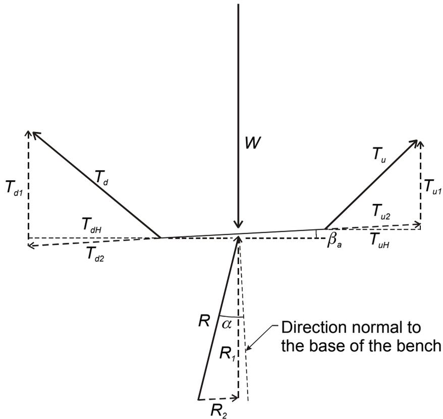
Figure 6. Decomposition of the forces acting on an anchor bench into vertical components (subscript 1) and components parallel to the base of the anchor bench (subscript 2).
