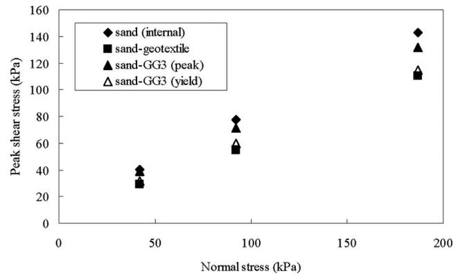
**Fig. 5.** Peak shear strength of Ottawa sand (internal), sand-geotextile interface, and sand-GG3 interface
