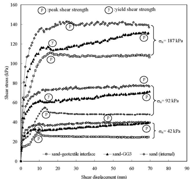
Fig. 3. Shear stress-displacement behavior of Ottawa sand, sand-geotextile interface, and sand-GG3 interface
