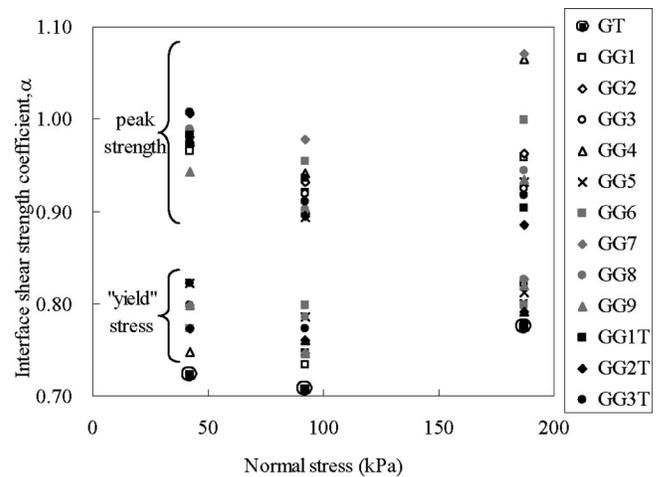
**Fig. 6.** Interface shear strength coefficient,  $\alpha$ , for the different sand-geosynthetic interfaces
