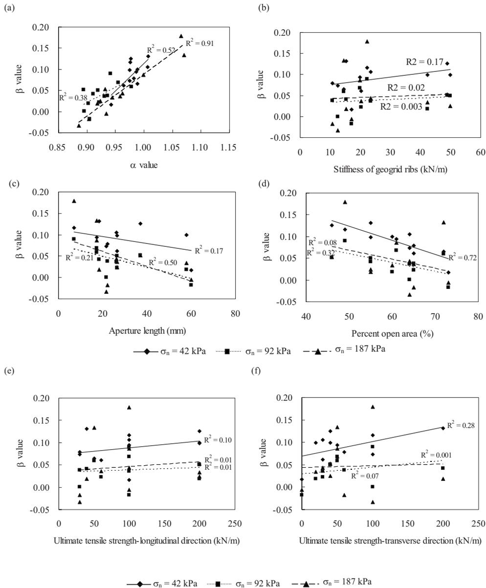
**Fig. 9.** Correlation of the passive resistance contribution ratio,  $\beta$ , with different parameters: (a) interface coefficient; (b) geogrid stiffness; (c) aperture length; (d) percent open area; (e) ultimate tensile strength in the longitudinal direction; and (f) ultimate tensile strength in the transverse direction
