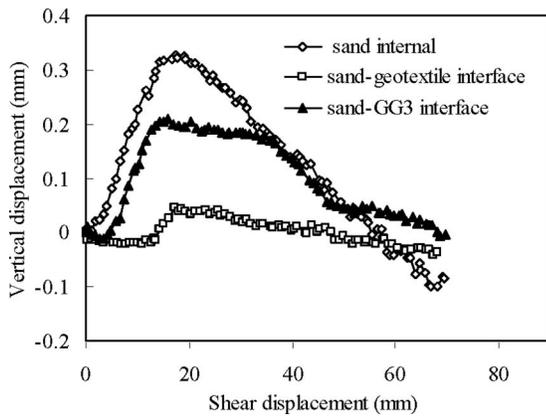
**Fig. 4.** Vertical displacement versus shear displacement results for direct shear tests of Ottawa sand (internal), sand-geotextile interface, and sand-GG3 interface
