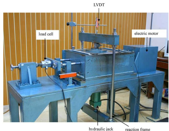
**Fig. 1.** View of large-scale direct shear apparatus
