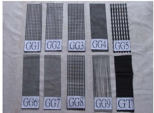
Fig. 2. Geosynthetic specimens used in this investigation
