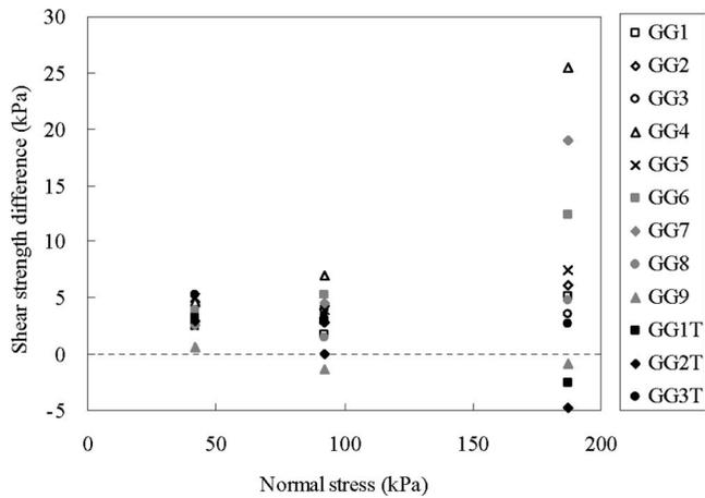
**Fig. 7.** Deviation of measured shear strength from value predicted by Eq. (3)
