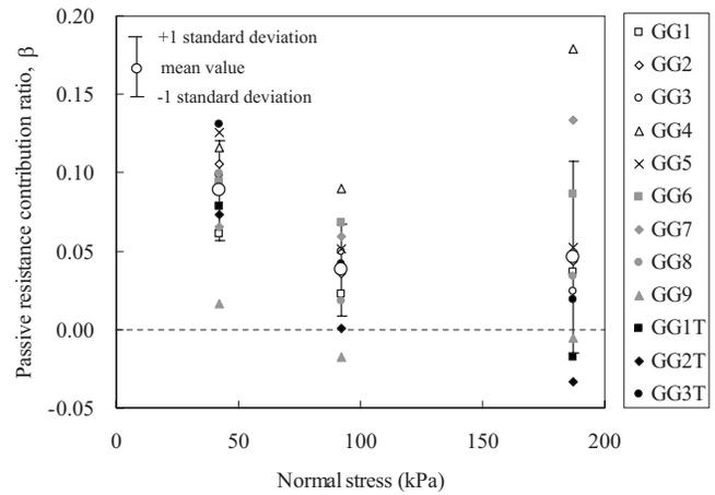
**Fig. 8.** Passive resistance contribution ratio,  $\beta$ , for different sand-geogrid interfaces
