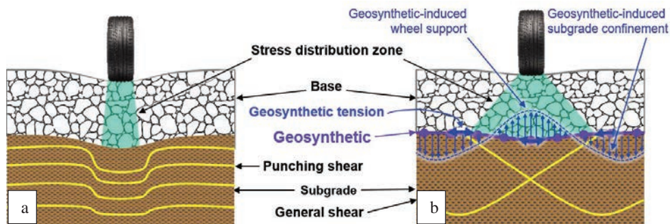
Fig. 5. Use of geosynthetics in stabilization of road subgrades: (a) roadway designed without geosynthetics, (b) roadway designed with geosynthetics.
