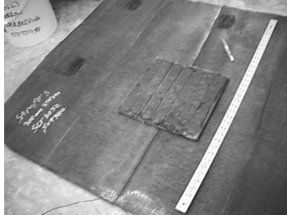
Figure 5: Specimen being trimmed to the dimension of the textured rigid substrate
