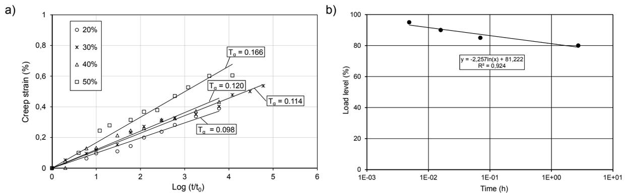
Figure 5 – Results from creep tests conducted with the biaxial woven geogrid: a) Conventional creep tests with specimens subjected to load levels from 20 to 50% of UTS; b) Conventional creep rupture curve obtained with specimens subjected to loads from 80 to 95% of UTS.
