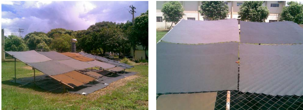
Figure 1. Geotextiles samples exposed to weathering.
