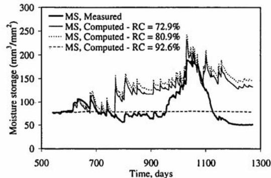
Figure 8: Variation in computed moisture storage for three densities
