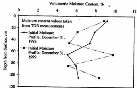
Figure 3: Initial soil moisture content data for model starting dates on January 1, 1999 (day 176) and January 1, 2000 (day 541)
