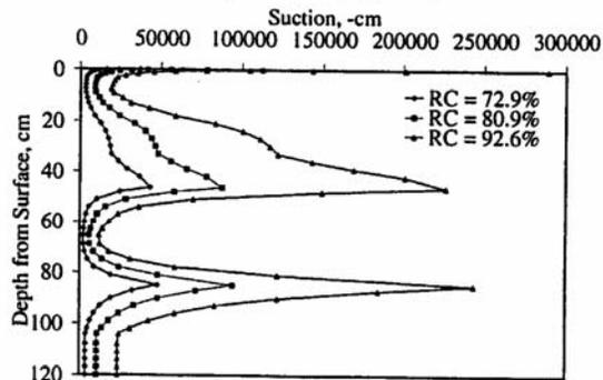
Figure 4: Initial suction data for a model starting date of January 1, 2000 (day 541)
