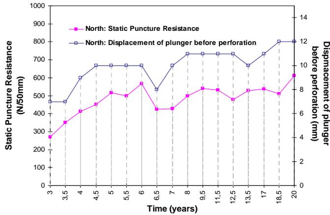
Figure 3. Variation of resistance to static puncture and the displacement of the plunger before perforation in north specimens.
