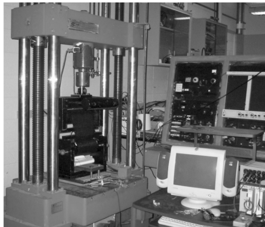
Fig. 8 Wide-width tensile test conducted with roller grips at the University of Texas at Austin
