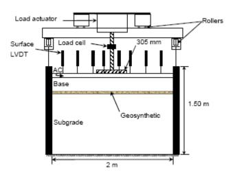
Figure 9: Cyclic plate load test (Perkins 1999)
