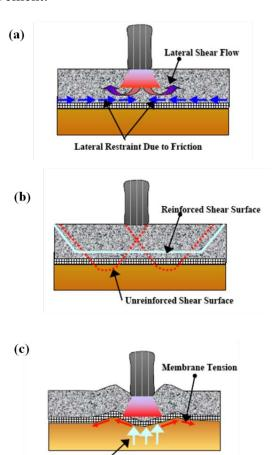
Figure 3: Reinforcement mechanisms induced by geosynthetics (Holtz et al. 1998): (a) Lateral restraint; (b) Increased bearing capacity; and (c) Membrane support
