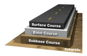
Figure 1: Cross-section of flexible pavement system (Muench 2006)
