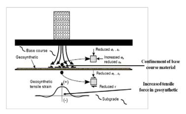
Figure 7: Mechanisms due to soil-geosynthetic interaction in geosynthetic- reinforced pavement that have been tried to be represented in laboratory tests (Perkins 1999)
