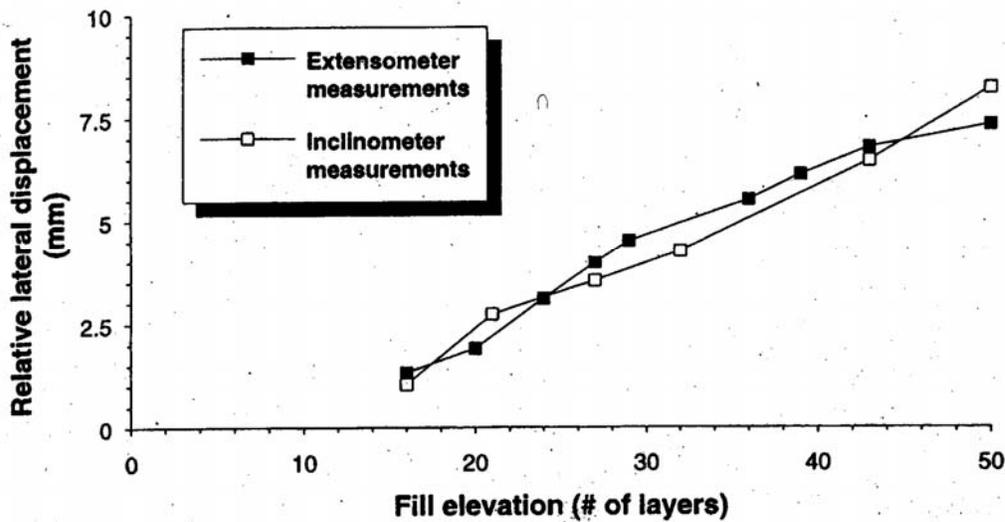
Figure 6. Development of relative displacements with increase in fill height (measured by inclinometers and extensometers).
