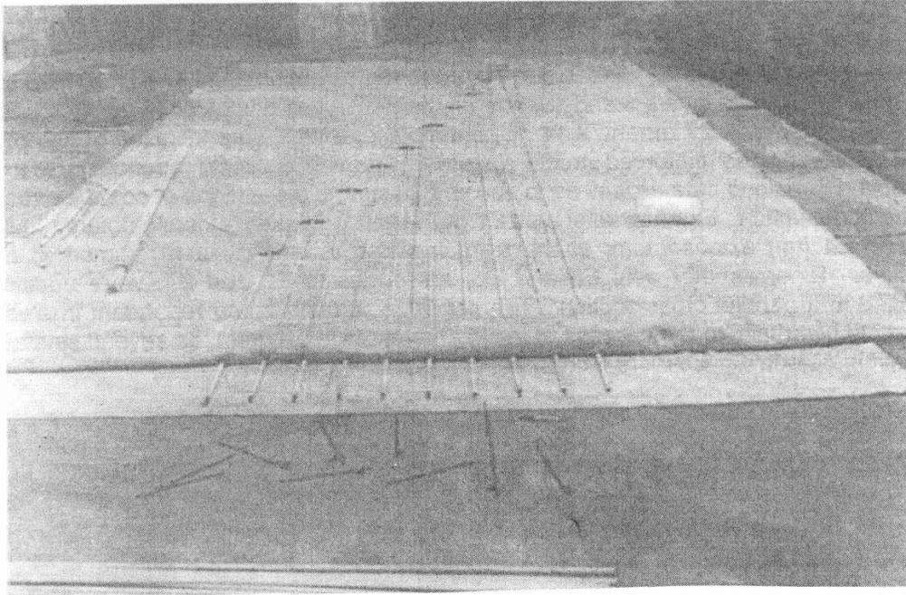
Figure 4. Geotextile layer instrumented with extensometers ready for placement in the field.
