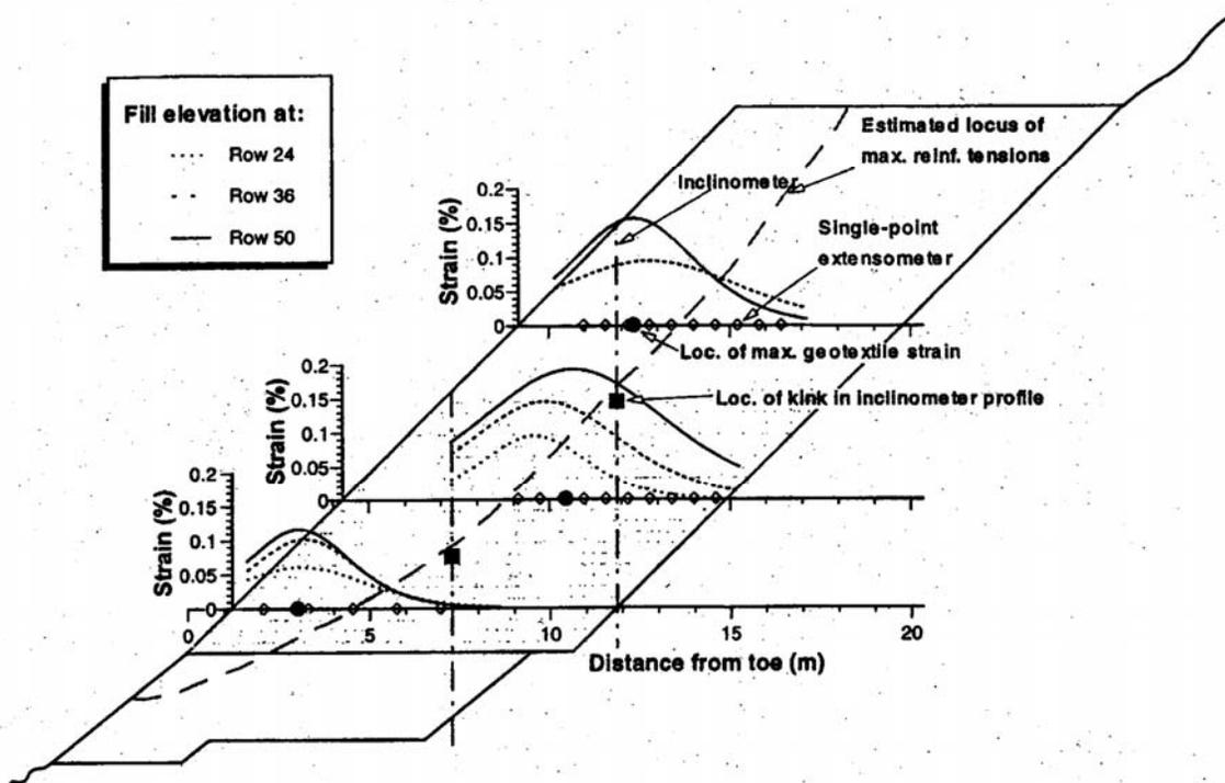
Figure 7. Distribution of strains during construction in each instrumented geotextile layer.
