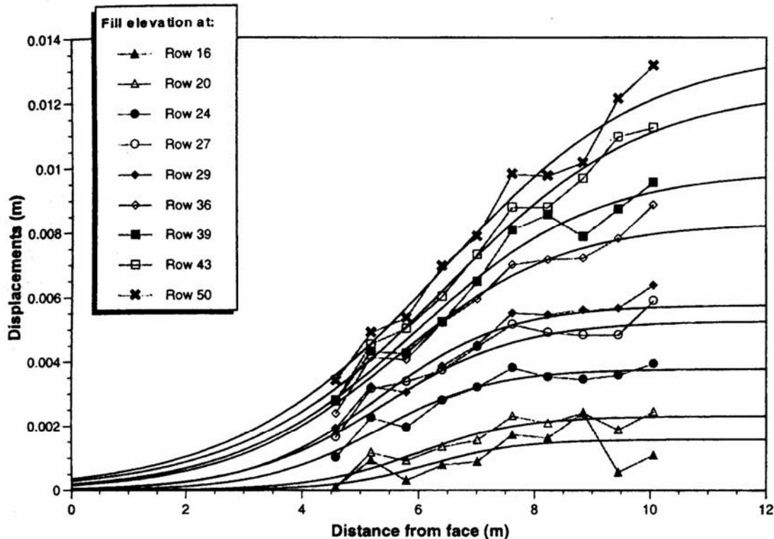
Figure 5. Lateral displacements measured by extensometers attached to geotextile layer 15 (Extensometer set E2)
