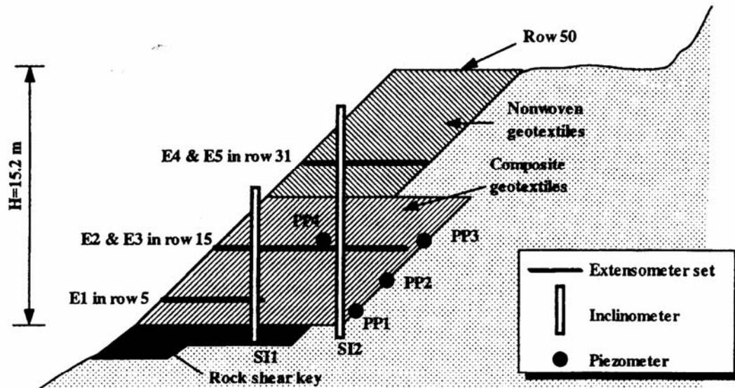
Figure 2. Cross section of the reinforced slope showing the instrumentation layout
