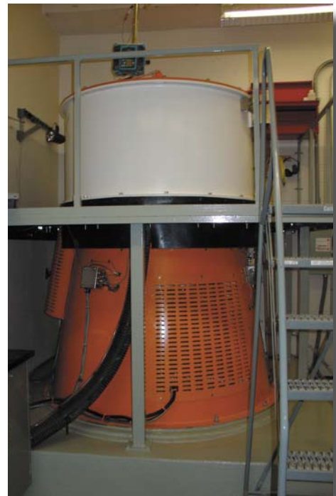
Above: A Smaller Conventional Centrifuge was Used to Manually Take Height and Weight Measurements During the Testing Process.
