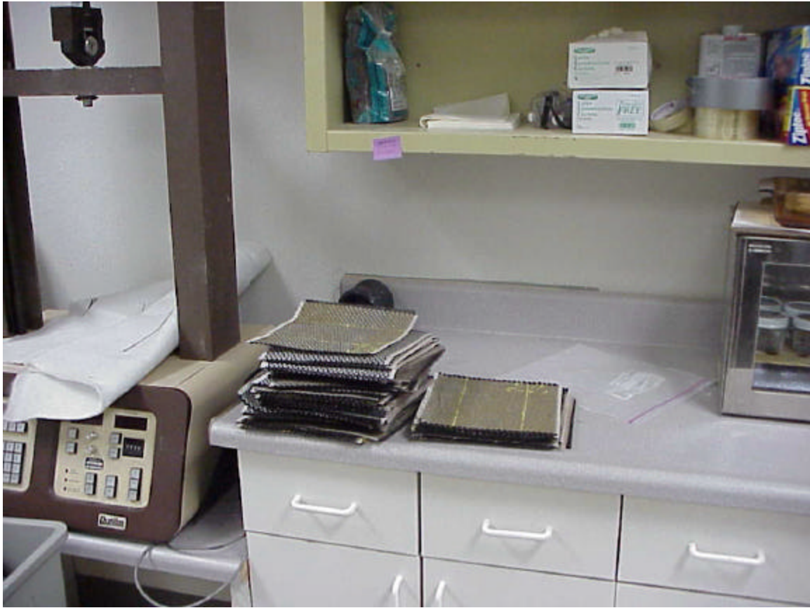
Photo 14. Fabric Specimens Ready for the Wide-Width Tensile Test (ASTM D 4595).
