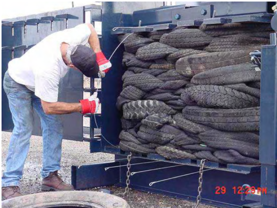
Figure D.40 Construction of tire bale 2001
