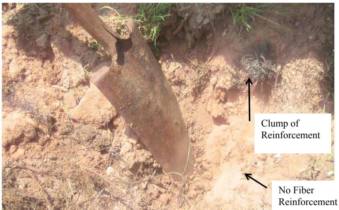
Figure D.55 Clumps of Fiber Reinforcements Located at Depth of About 1 Ft.
