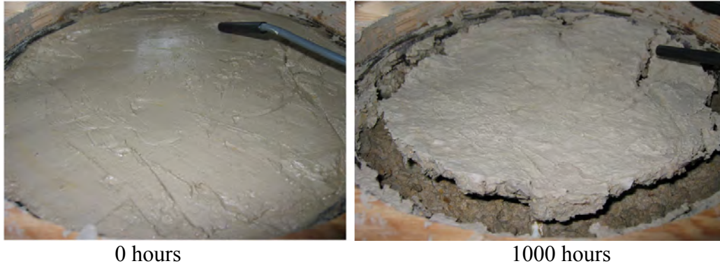
Figure 4.26: Surface of Soil Column 3 before and after second drying phase
