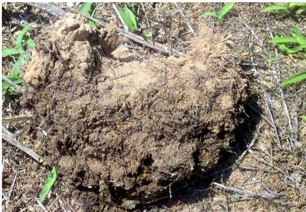
Figure D.57 Large Clump of Dark Clay Material with Fiber Reinforcement Excavated from About 1 Ft.
