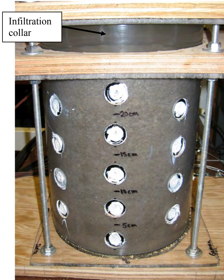
Figure 4.18: Infiltration setup for Soil Column 3
