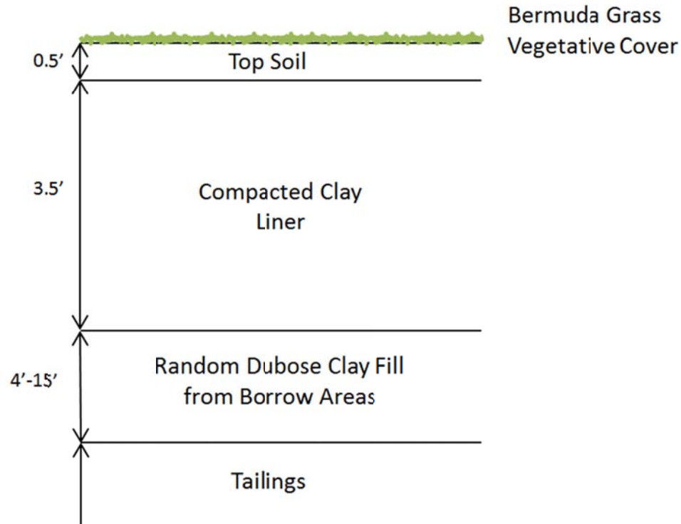
FIGURE 10 – Cross Section of Final Cover
