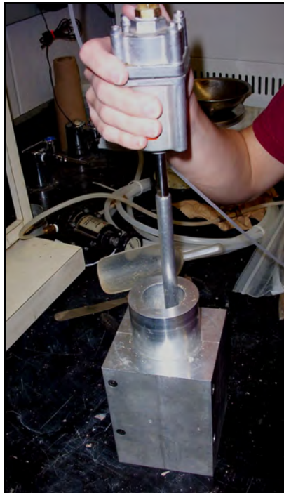
Figure 4.4: Compaction of specimen using the Marsh-Bellofram actuator air piston.
