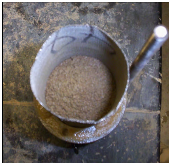
Figure 4.9: Top view of specimen in a specimen holder before trimming.
