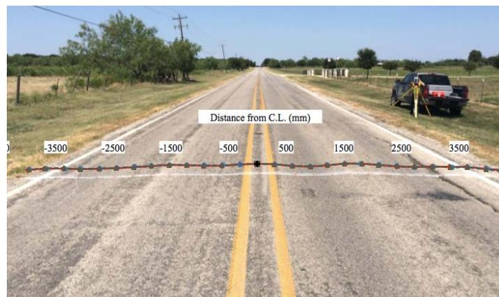
**Fig. 7.** Total station survey of the marked sections in the field
