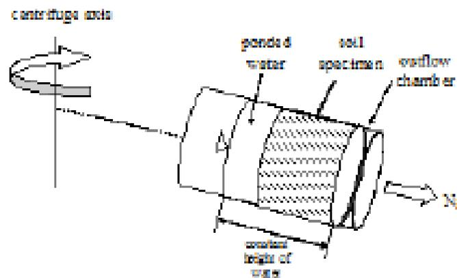
**Fig. 14.** Schematic of centrifuge test setup
