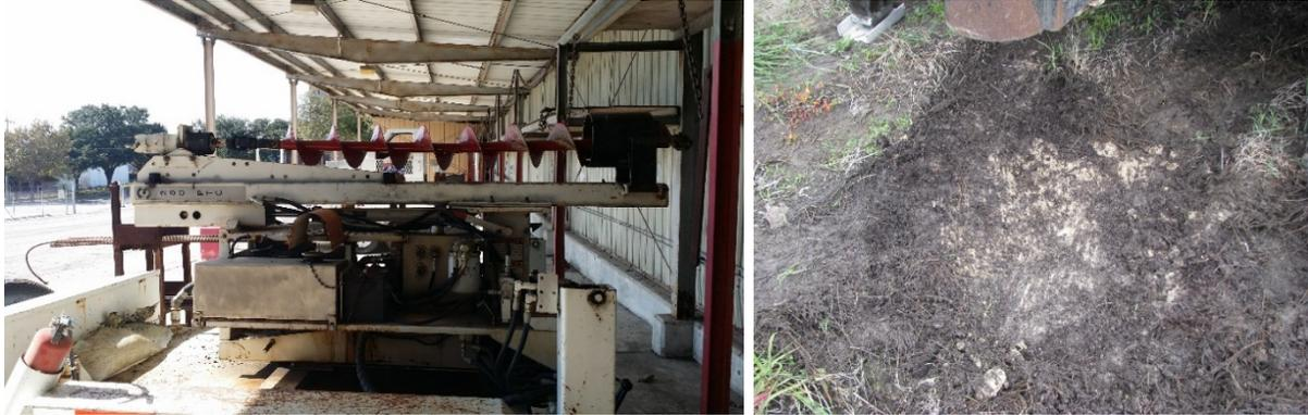
**Fig. 10.** Continuous flight auger and soil surface cleared of vegetation
