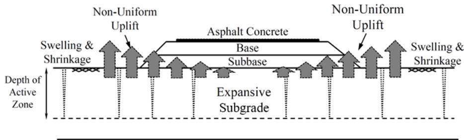
**Fig. 3.** Non-uniform environmental loading imposed on road structures by expansive subgrades
