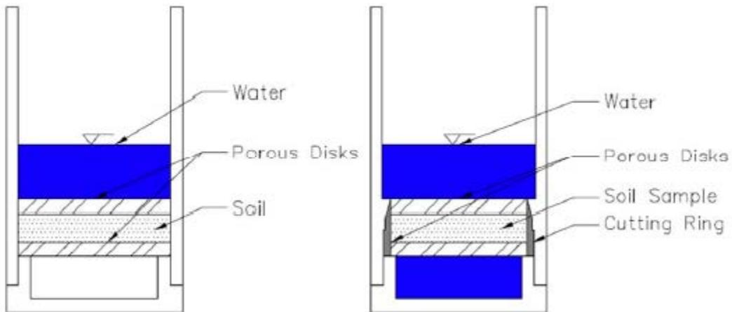
**Fig. 13.** Schematic of single and double infiltration setups
