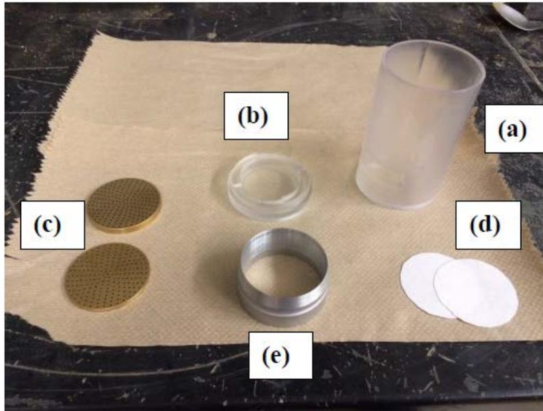
**Fig. 12.** Layout of double infiltration setup: (a) top cup; (b) base cup; (c) porous disks; (d) filter papers; (e) cutting ring
