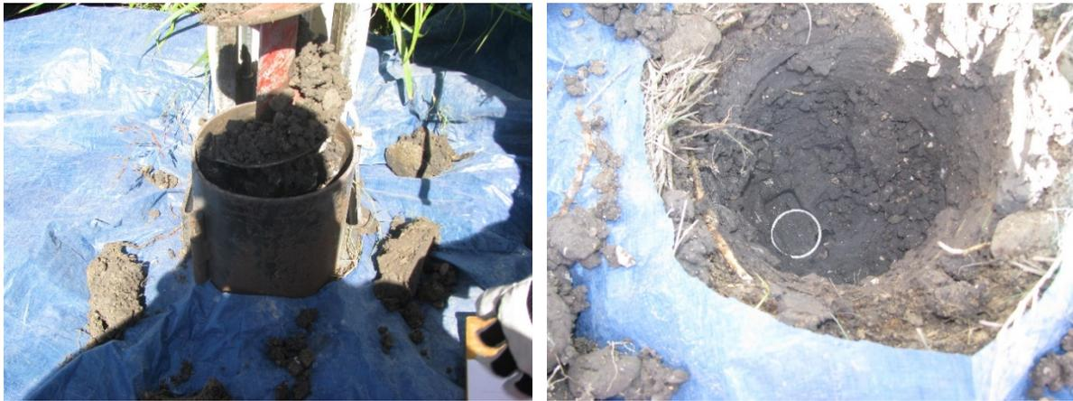
**Fig. 11.** Soil cuttings being removed from tarp-covered borehole and cutting ring for density sample
