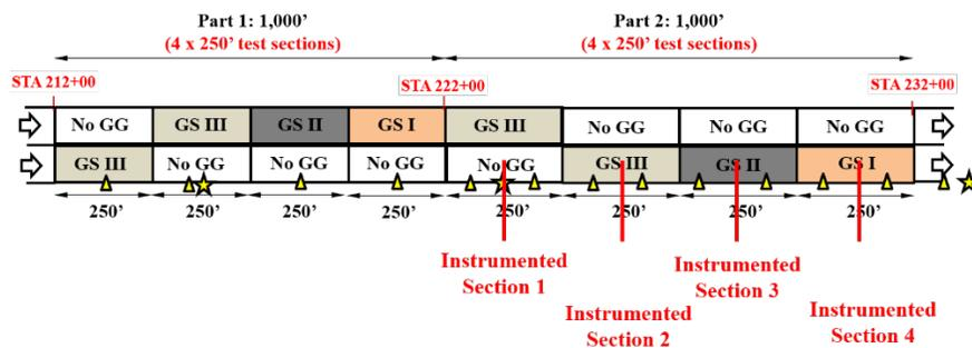
**Fig. 47.** Example design of test sections
