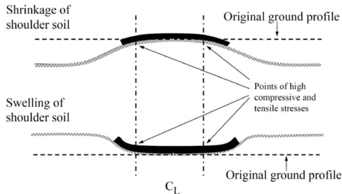
**Fig. 4.** Conceptual model for generating environmentally induced longitudinal cracks in pavements (Gupta et al. 2008)
