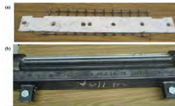
Figure 2.4: Clamping system (a) Original design consisting of plastic sheets (b) Modified design with roller grips.
