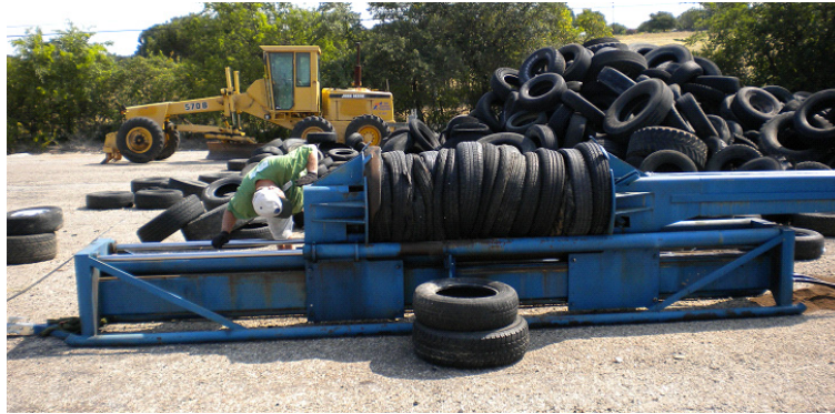
Figure 2.9: Compression of the Whole Scrap Tires into the Cylinder Tire Bale
