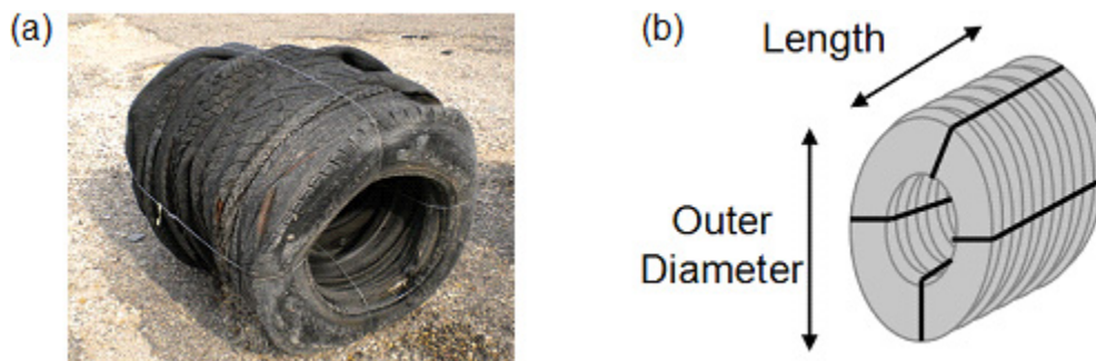
Figure 2.10: (a) Photograph of a Cylinder Tire Bale and (b) Illustration of the Cylinder Bale Dimensions
