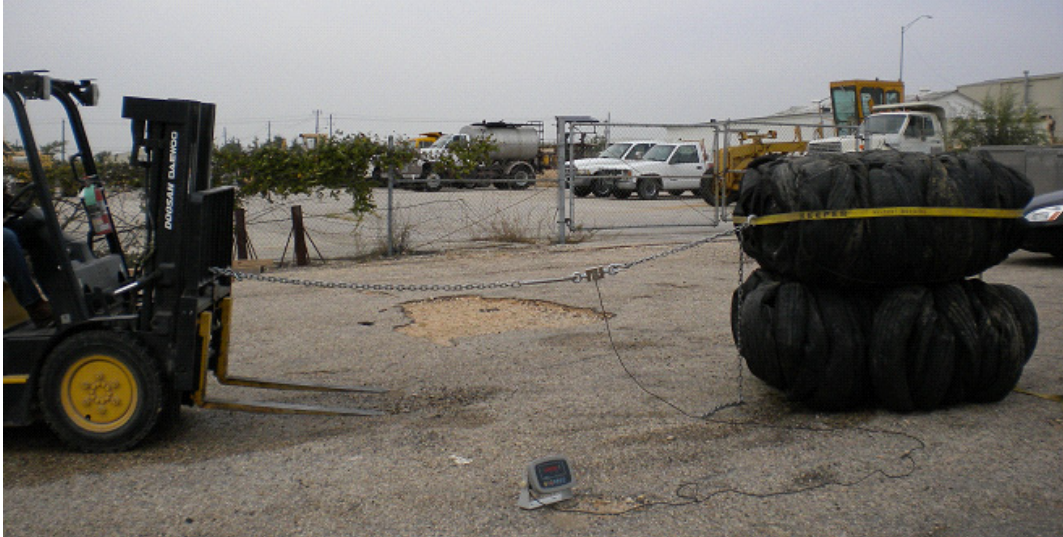
Figure 3.5: Field Direct Shear Test for the Site 2 Block Tire Bales
