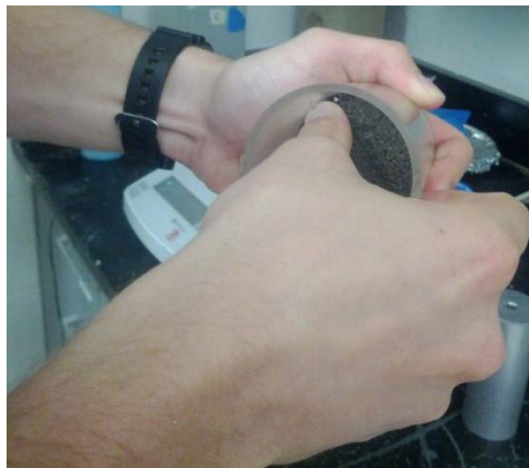
Figure 3: Densification of Soil Using Thumb
