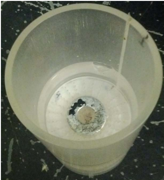
Figure 9: Final Permeameter Cup Assembly with 2 cm of Ponded Water Head and Overburden Washer
