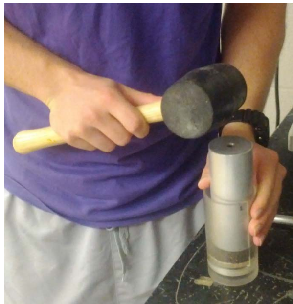
Figure 5: Compaction of Soil Specimen Using Rubber Mallet and Large Diameter Compaction Rod
