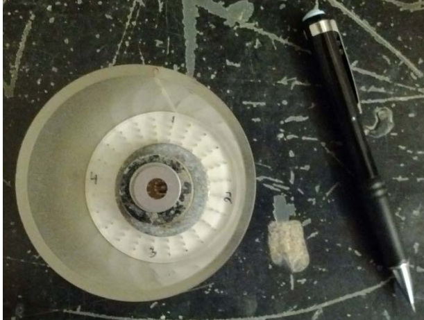
Figure 7: Assembled Permeameter Cup with Overburden Washers and Washers Simulating 51.3 Grams of Overburden from the Poned Water
