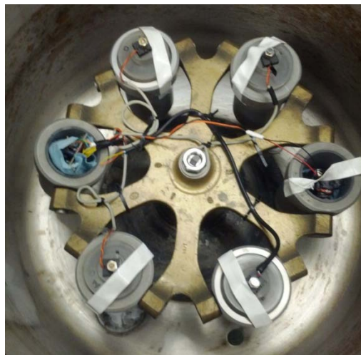
Figure 8: Assembled Testing Setup within the Centrifuge
