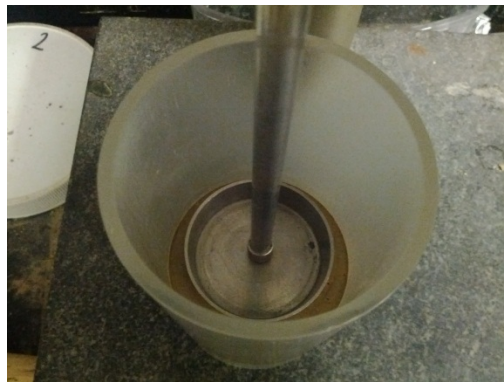
Figure 6: Measurement of Compacted Specimen Using Metal Plate and Mounted Caliper
