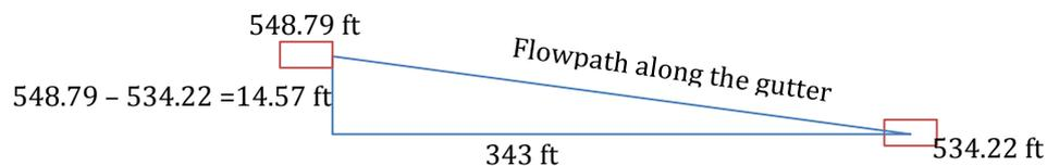
$$\text{Slope} = \frac{14.57}{343} = 0.0424 \frac{\text{ft}}{\text{ft}}$$
