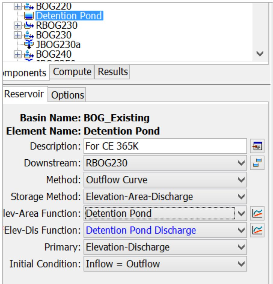
Now if you save the model and run HEC-HMS you can see the effect of the detention pond on various storm intensities. You can change the outlet structure design and see if this has an effect. When I first ran this modified model it did not work but I closed HEC-HMS and reopened it and ran the model and it worked fine.
