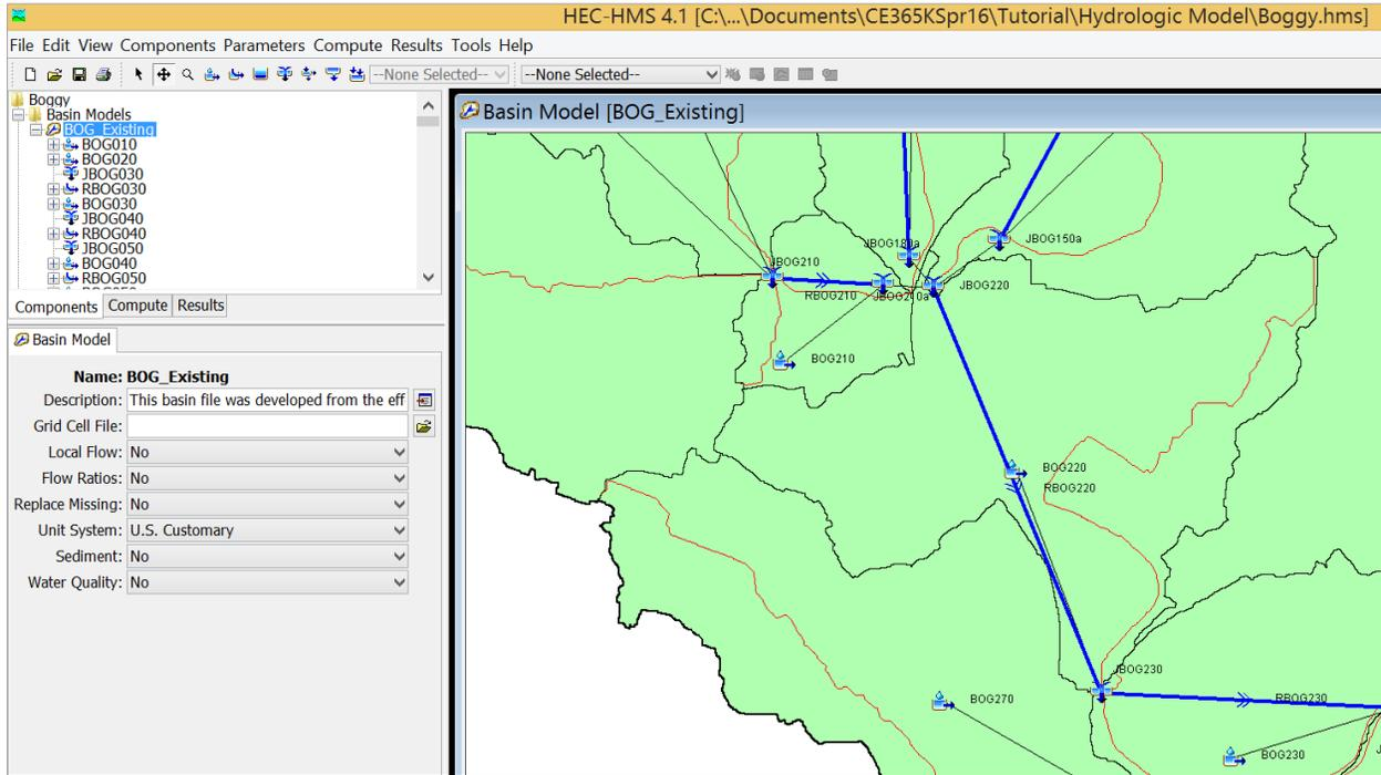
Right click on the JB230 junction and select **Cut Element**. In HEC-HMS select the Create Reservoir Tool
