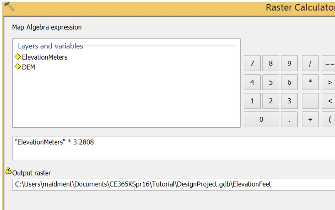
Now we have an elevation raster with values from Elevation 471 to 495 ft
