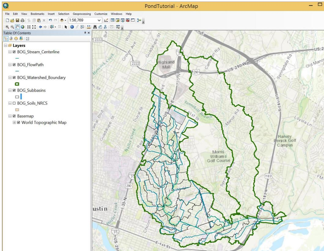
Right click on the **Subbasin** feature class, select **Properties** and set the Label field as **Subname** with size **12**. Right click on the Subbasin feature class again and select Label Features so you can see which subbasins you are dealing with.
