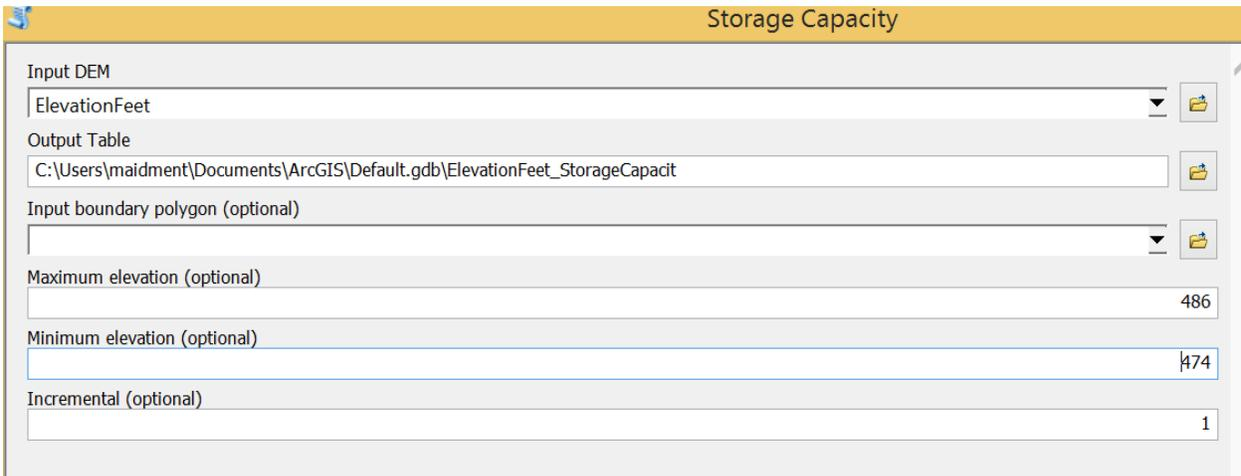
Open the resulting Storage Capacity table and you'll see Area in m<sup>2</sup> and Volume in m<sup>2</sup>-ft as shown below indexed by 1 foot increments of elevation as we need.
