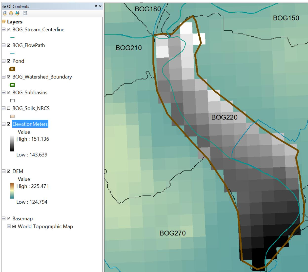
This is an elevation model with cells that are 30m x 30m in size and elevations in meters. Lets convert the elevations into feet. Search for “Raster Calculator” under the Search Tab in ArcMap, create the expression “DEM” \* 3.2808 and store the results as **ElevationFeet**, as shown below.
