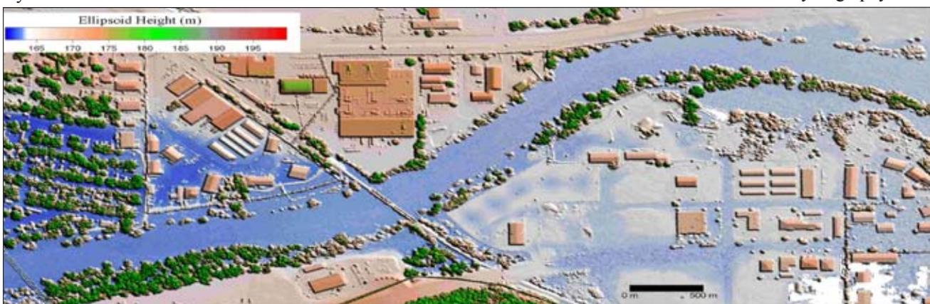
Color coded map of flood water surface elevation using lidar in Iowa City, Iowa. High-resolution lidar data can be used to calculate more accurate base flood elevations and delineate floodplain boundaries to reduce future flood losses. Ellipsoid height is a measure of elevation. SOURCE: Courtesy of Ramesh Shrestha, University of Florida, and Witold Krajewski, IIHR-Hydroscience and Engineering, used with permission.
