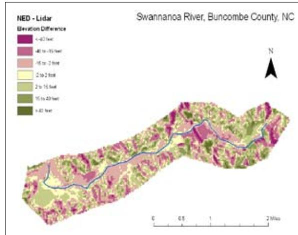
Elevation differences between the USGS National Elevation Dataset and lidar data, Swannanoa River, North Carolina. Areas in red and pink are lower than appear on FEMA flood maps and suggest that the floodplain extends further than expected. SOURCE: Courtesy of T. Langan, North Carolina Floodplain Mapping Program, used with permission.
