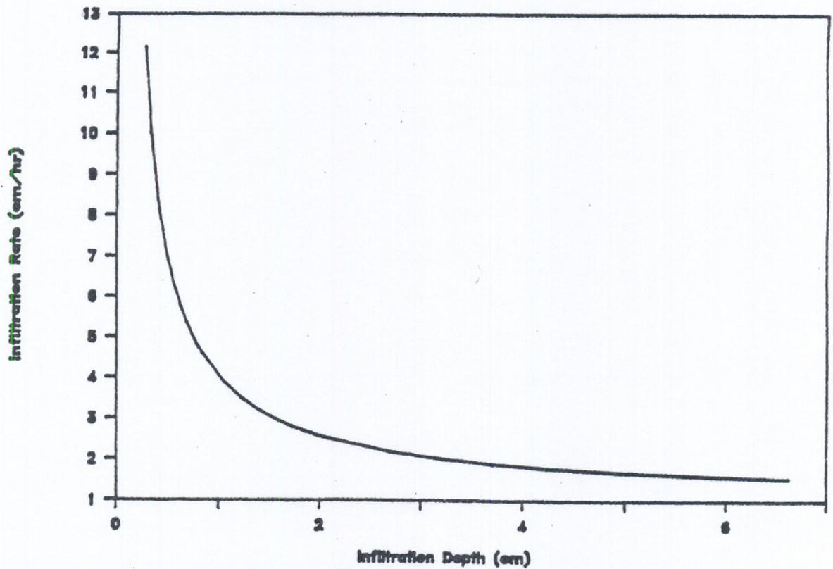
Fig. 4.3.2. Infiltration rate and cumulative infiltration depth computed by the Green-Ampt method.
