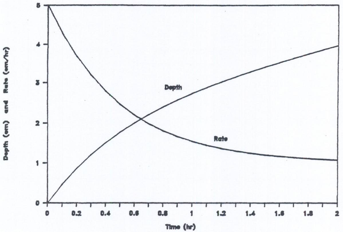
(b) Rate vs. Infiltration Depth
