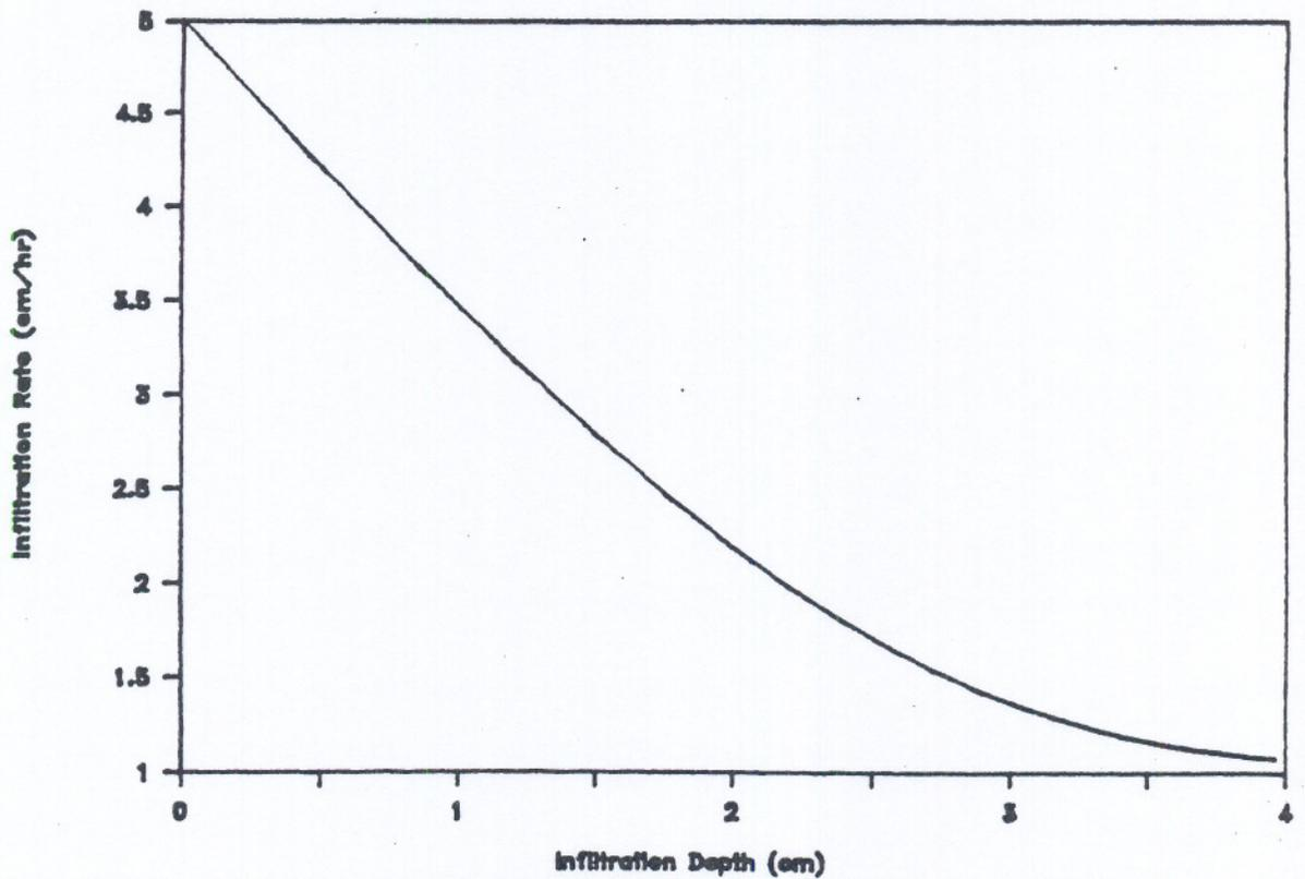
Fig. 4.2.3. Infiltration rate and cumulative infiltration depth computed by Horton's equation.
