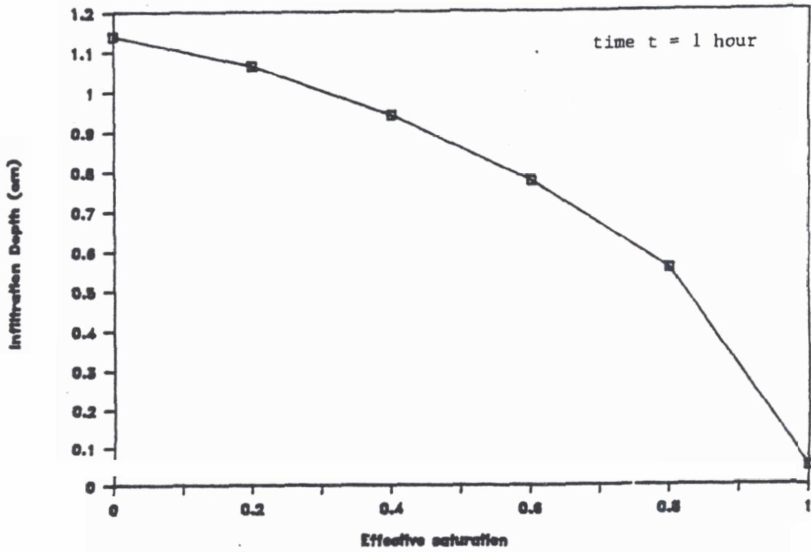
Fig. 4.3.4. Cumulative infiltration depth, computed by the Green-Ampt method, as a function of the initial effective saturation of the soil.
