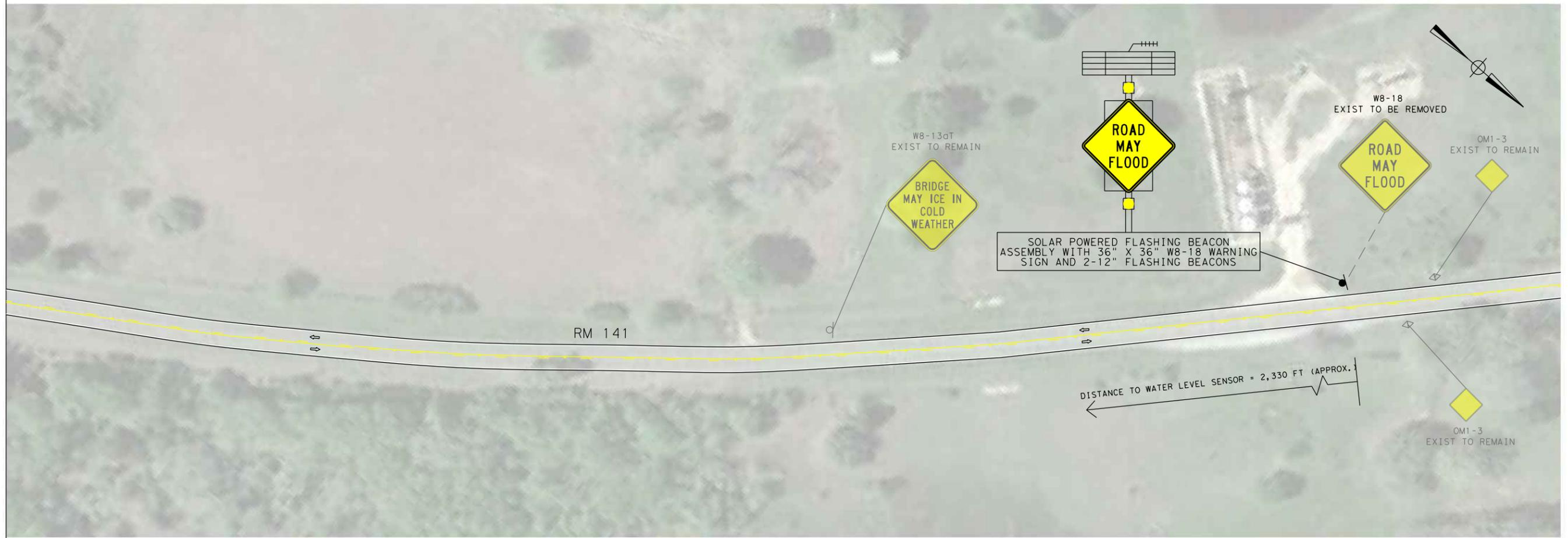
SOLAR POWERED FLASHING BEACON ASSEMBLY WITH 36" X 36" W8-18 WARNING SIGN AND 2-12" FLASHING BEACONS
