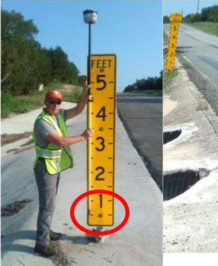
Pipe Information – One survey spot is acquired at the center of each pipe/culvert on both the upstream and downstream face.
