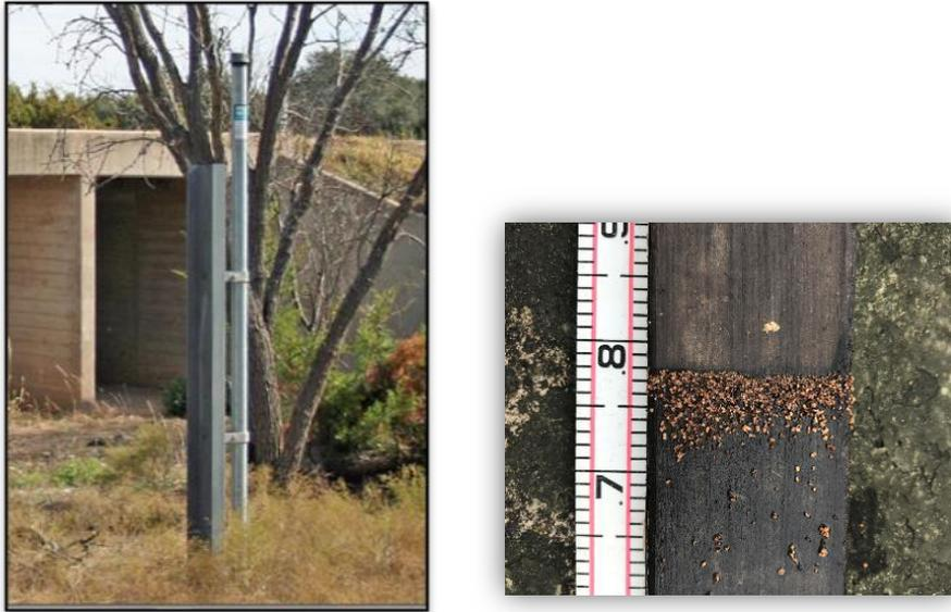
*Figure 3.3.4 Example of a crest stage gauge for measuring peak stage*
