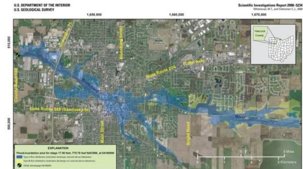
FIG. 3. Flood-inundation areas for Blanchard River near Findlay, Ohio (station 04180000), for type-A and type-B flow distributions, stage of 17.06 feet.
